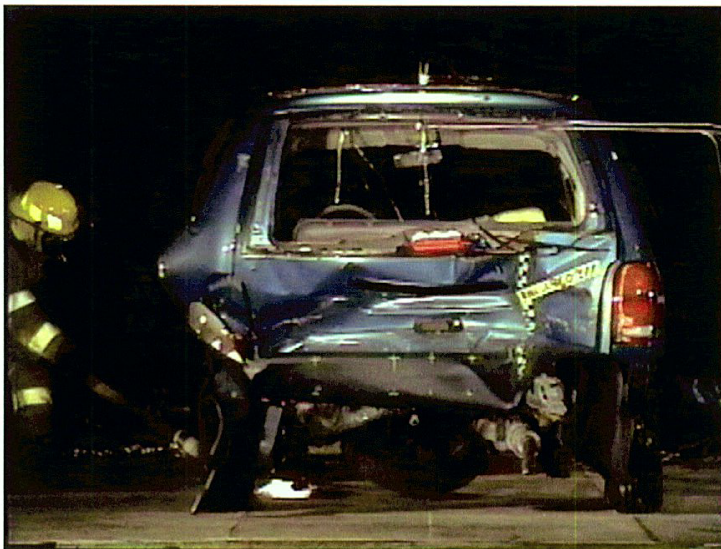
Figure 4. Fire Test F961116. Video still from Camera 1 showing ignition of the gasoline pool from the rear of the test vehicle.
