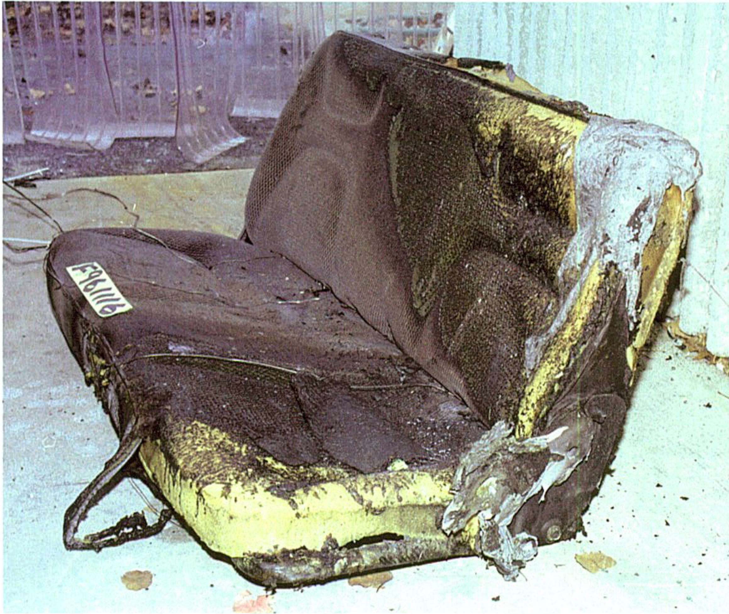
Figure 39. Fire Test F961116. Photograph showing fire damage to the seating areas of the second bench seat.
