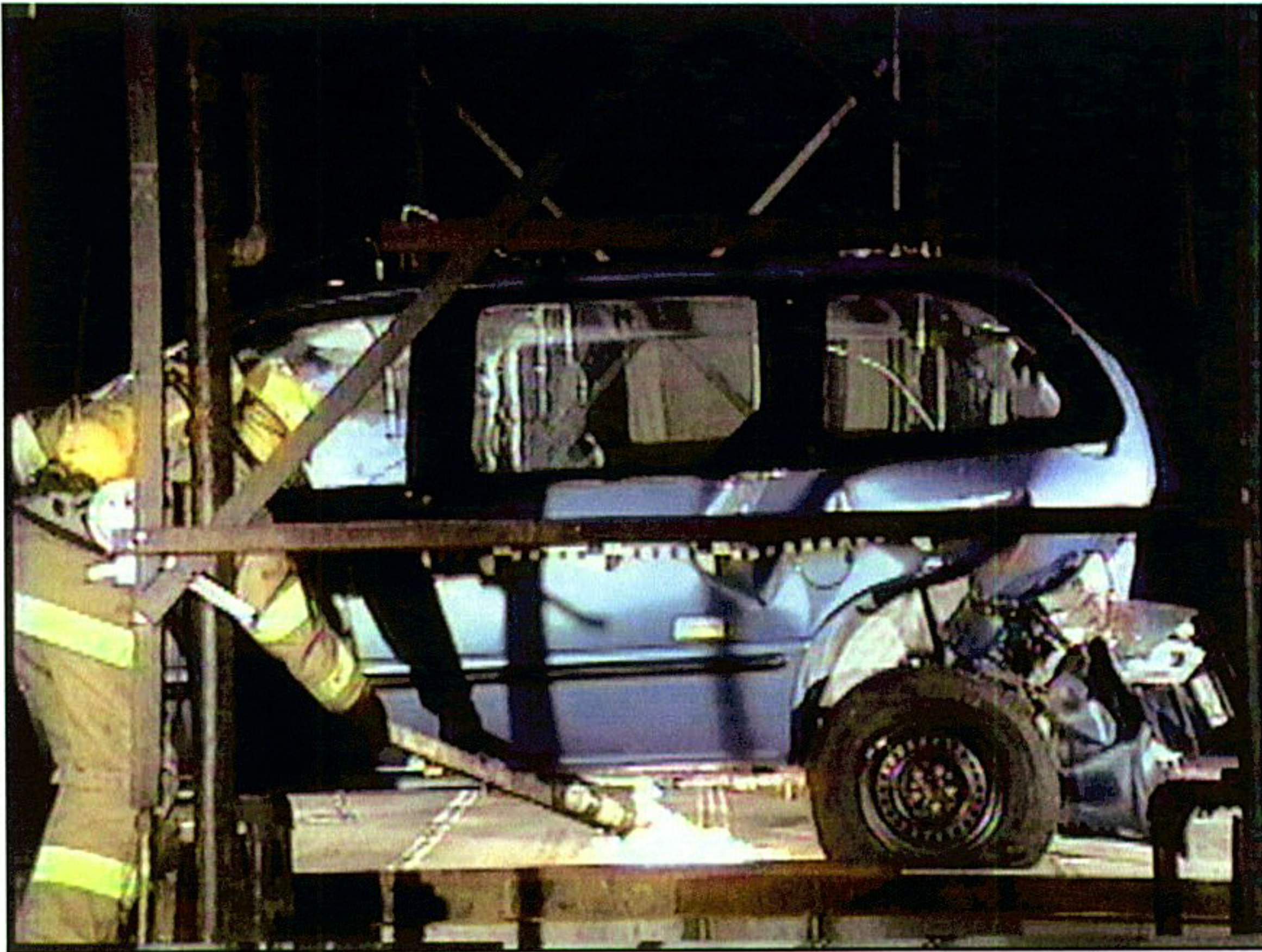
Figure 5. Fire Test F961116. Video still from Camera 2 showing ignition of the gasoline pool from the left side of the test vehicle. The structure in the foreground is the support for a fire suppression system located above the test floor.
