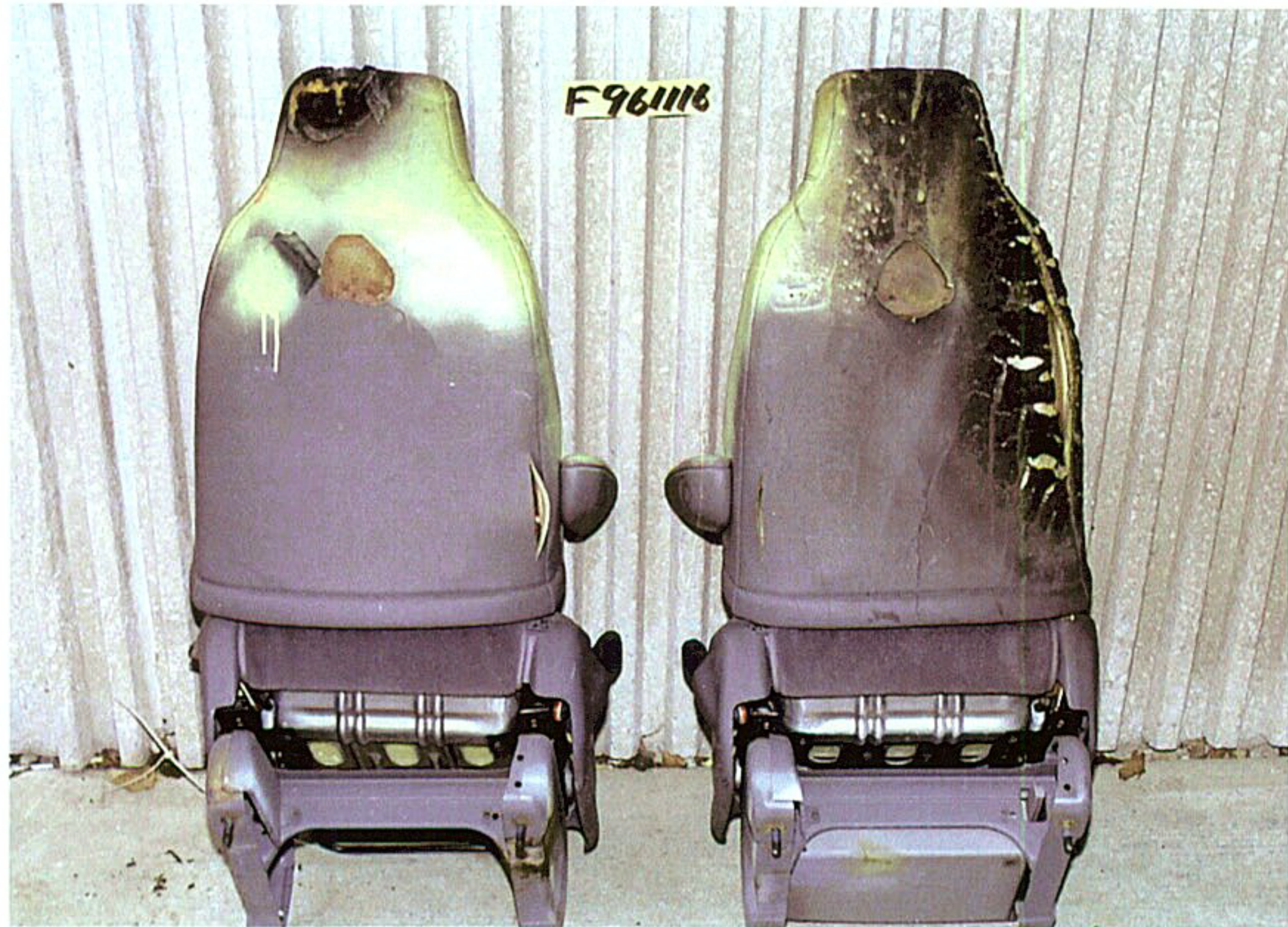
Figure 44. Fire Test F961116. Photograph showing fire damage to the driver's and front passenger's seats. (The yellow paint on the upper sections of the back panels and holes in the back panels were present when the test vehicle was received from Transportation Research Corporation.)
