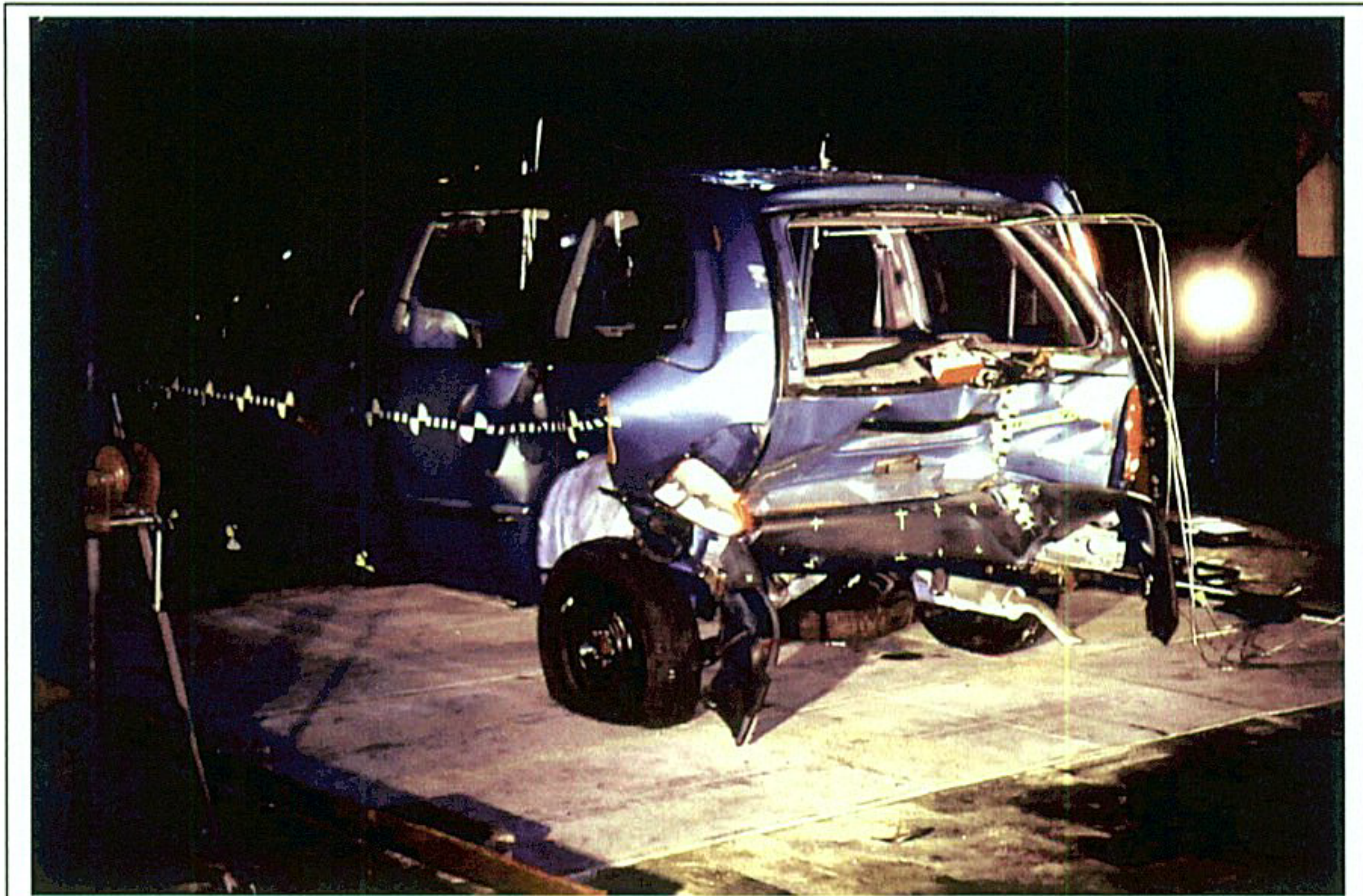
Figure 3. Fire Test F961116. Photograph of the test vehicle in position in the fluid containment pan before the fire test.
