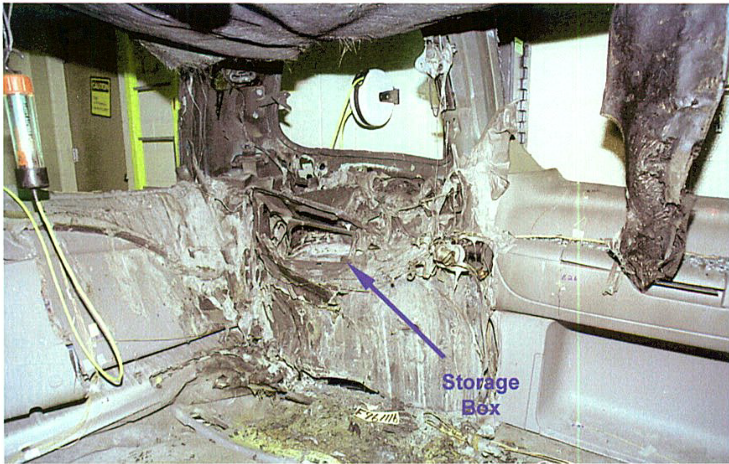
Figure 42. Fire Test F961116. Photograph showing the rear left corner of the passenger compartment of the test vehicle after this fire test. The storage box was not completely consumed by fire.
