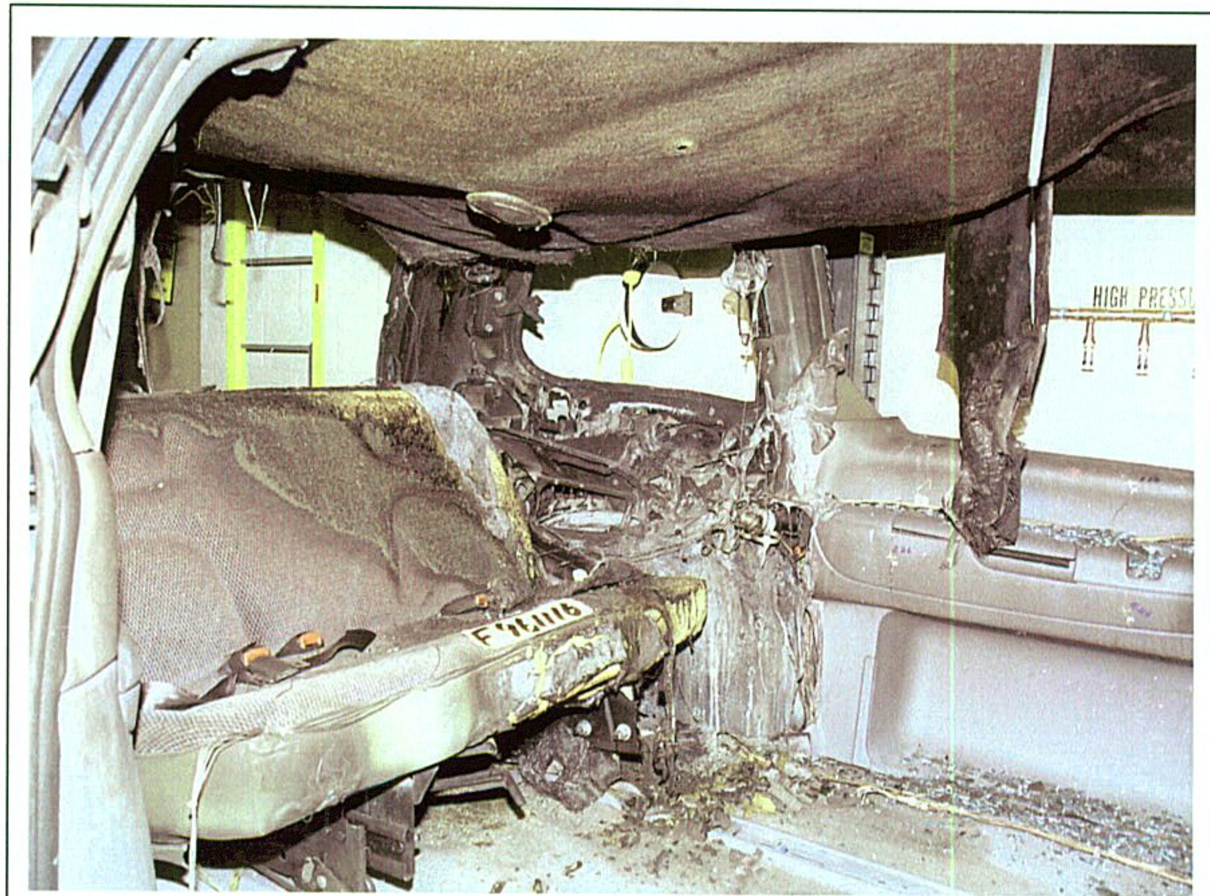
Figure 36. Fire Test F961116. Photograph showing fire damage to the second bench seat, the left quarter trim panel, the C- and D-pillar trim panels, and the headlining.
