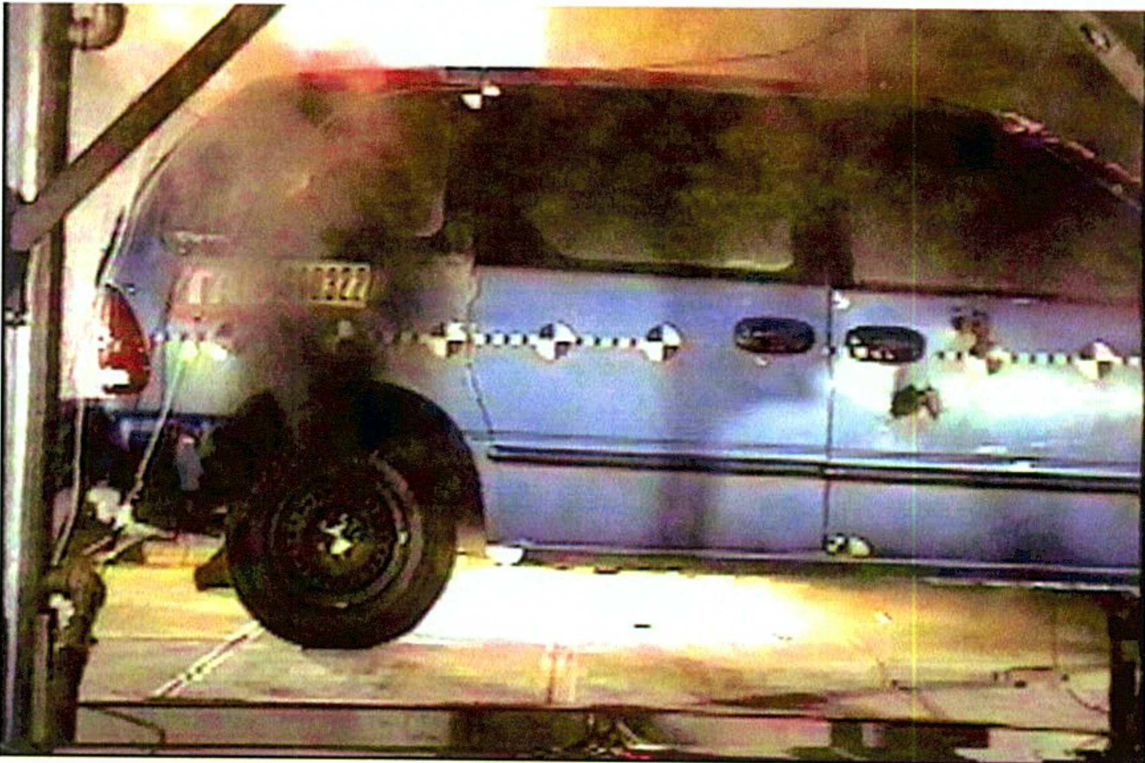
Figure 8. Fire Test F961116. Video stills from Camera 4 showing the right side of the test vehicle at 80 (upper panel) and 200 (lower panel) post-ignition. The diameter of the burning fuel under the vehicle was approximately 40 cm at 80 seconds post-ignition and approximately 80 cm at 200 seconds post-ignition.
