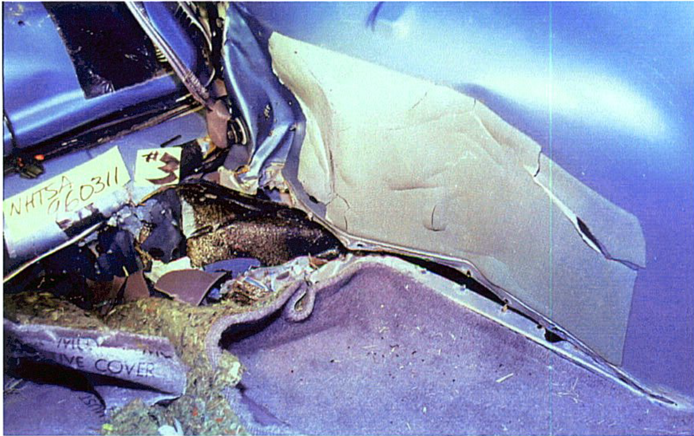
Figure 2. Fire Test F961116. Interior view of the left rear wheelhouse, floor pan, and lift gate of the test vehicle. The torn spot weld seams between the wheelhouse and the floor pan and the inner and outer wheelhouse panels are shown here. The second bench seat and interior trim were removed for this photograph.
