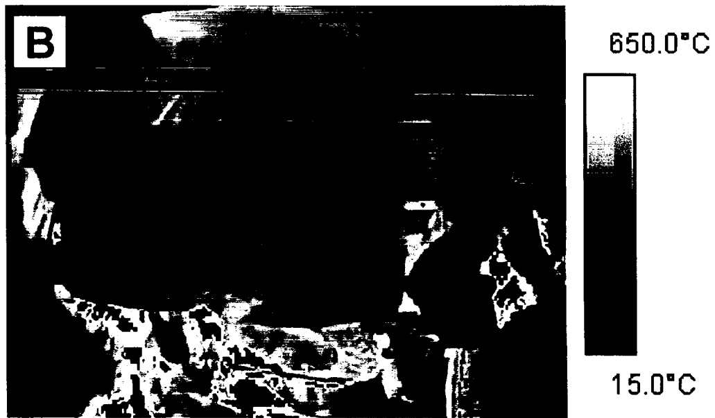
Figure 31. Fire Test F980609. Video still from Video Camera 1 (A), Infrared thermogram from IR3 (B), video still from Camera 4 (C), and Infrared thermogram from IR4 (D) at 157 seconds post-ignition.
