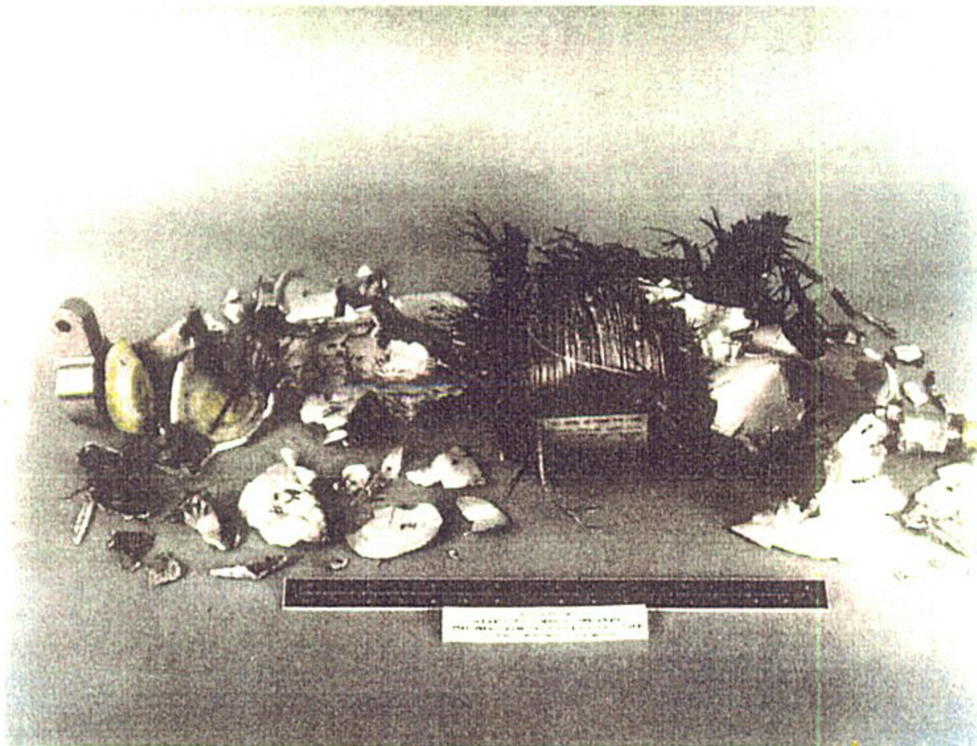
Figure 9. COPV Failed Upon Impact
