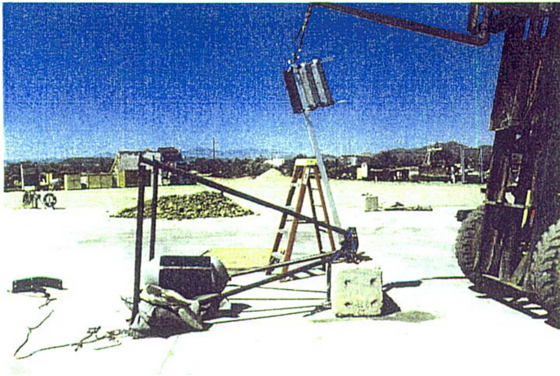
Figure 62. Impact Test Facility Just Prior to Impact of Tank 018
