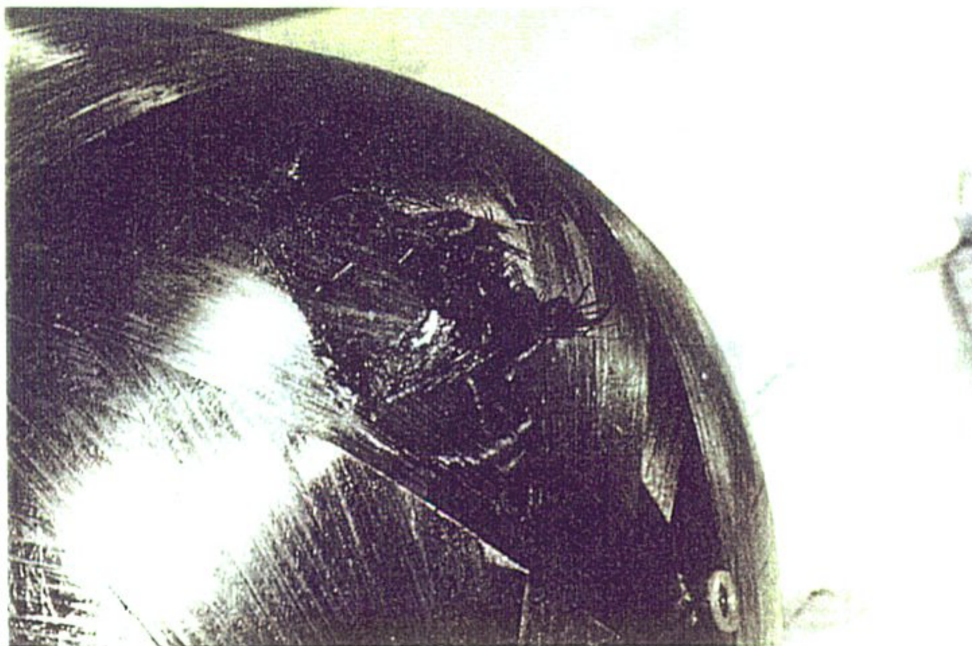
Figure 85. Failed Area on Tank 003, Close-up
