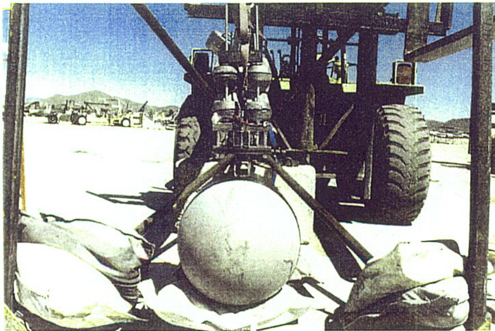
Figure 61. Large Impact Fixture Set-up for Tank 018, End View
