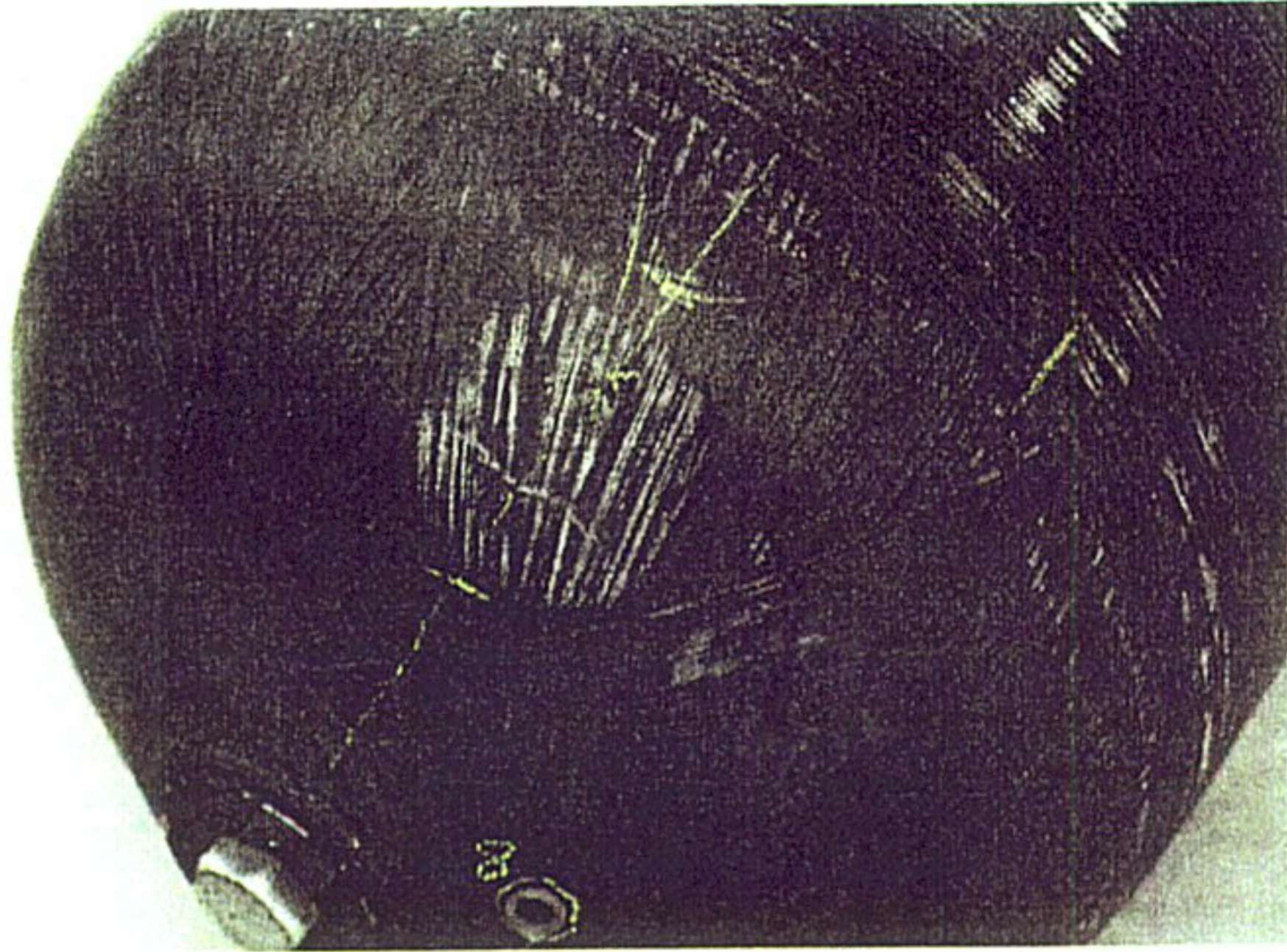
Figure 80. Impact Site on Tank 003
