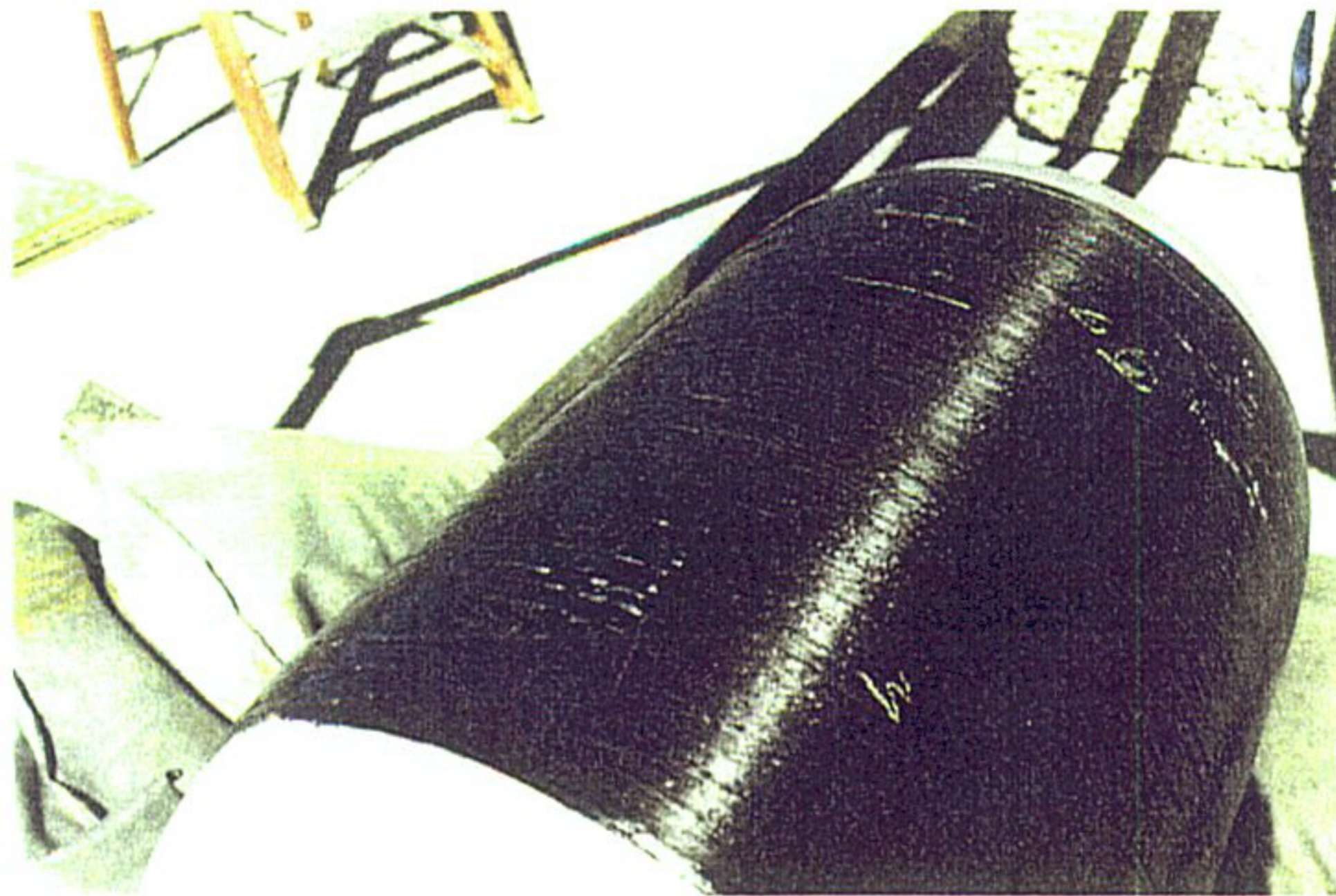
Figure 63. Post-Impact Damage on Tank 018, Overall View
