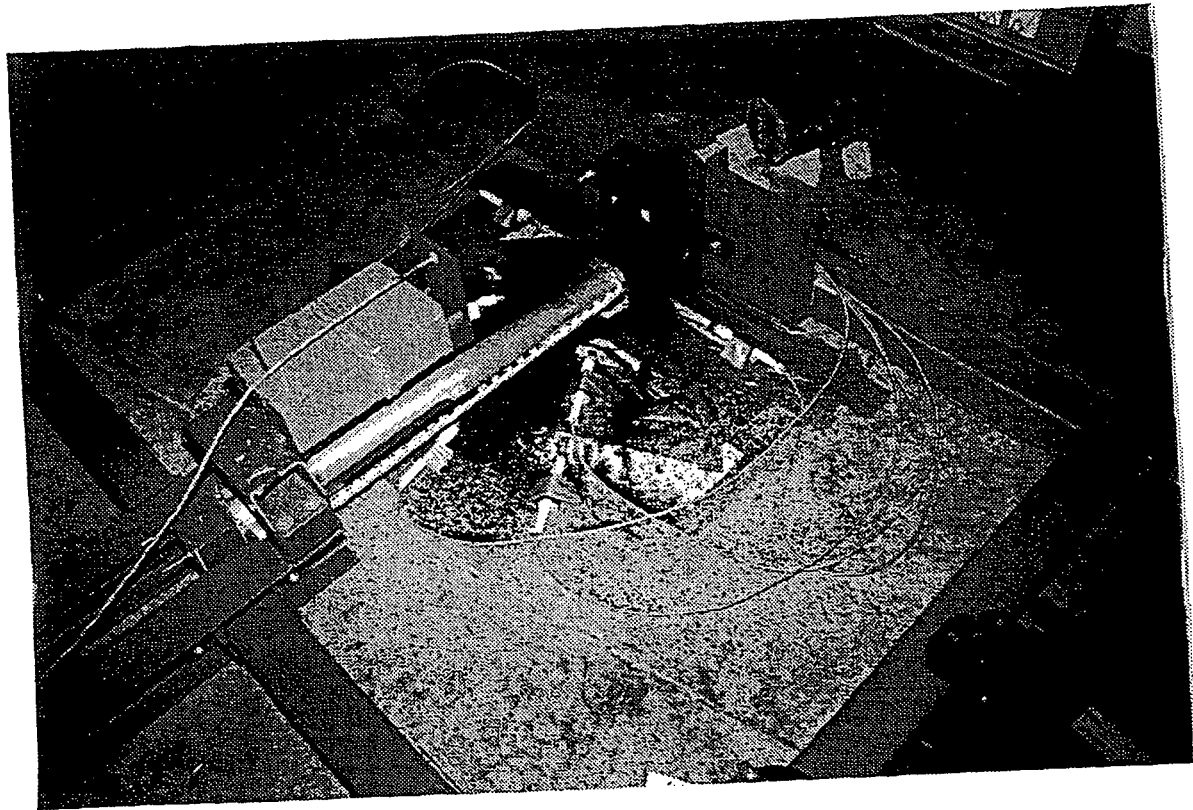
Canister #23: Wide Side Impact Slow Loading Method
