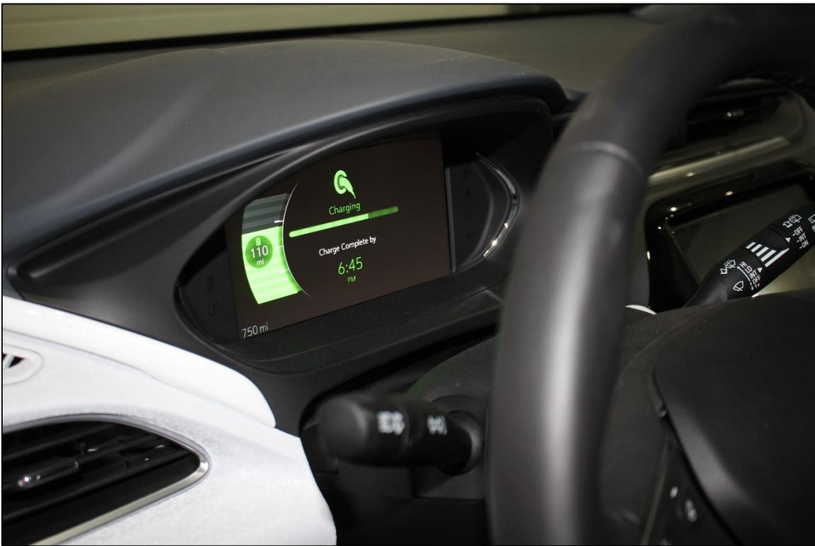
*Figure 50: Over-Current Pre-Test Instrument Cluster Message*
