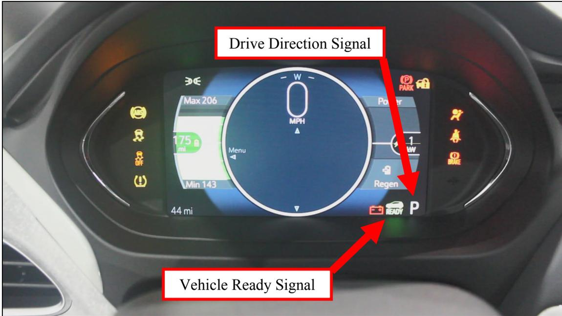
Figure 7: Vehicle Instrument Cluster
