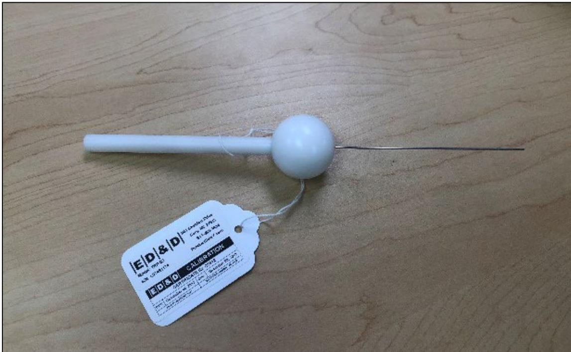
Figure 2: IPXXD Test Probe
