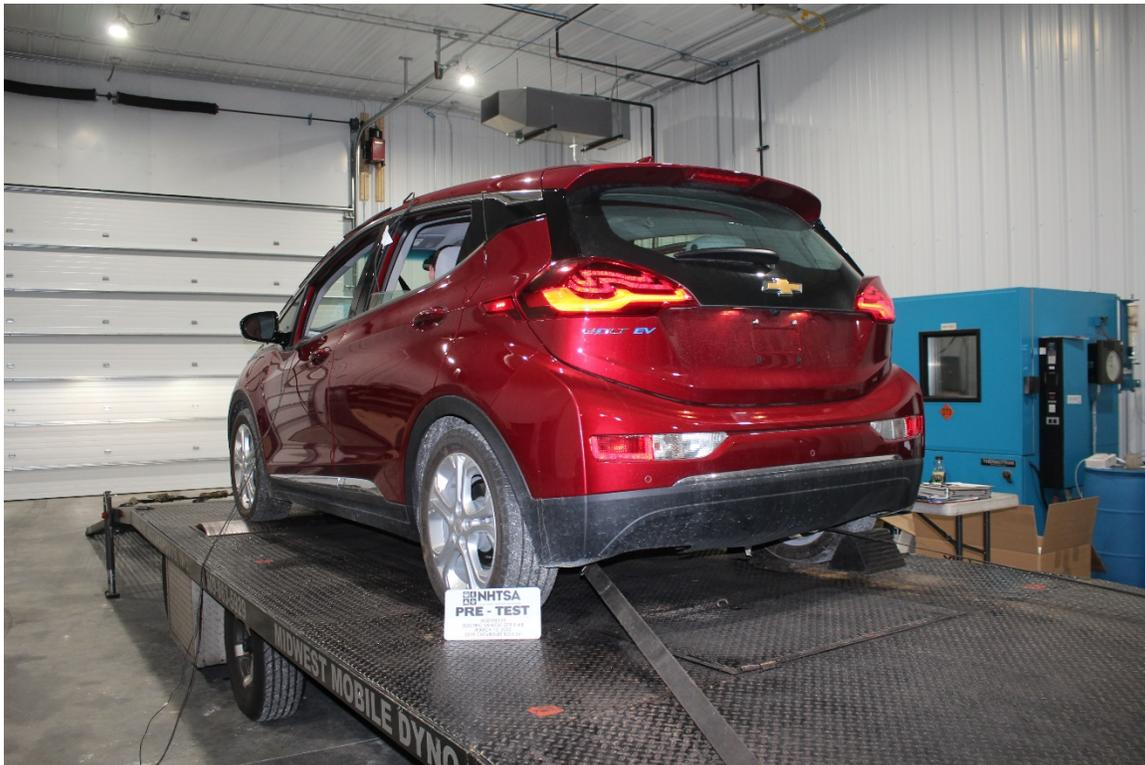
*Figure 38: Vehicle Installed on Mobile Dynamometer*
