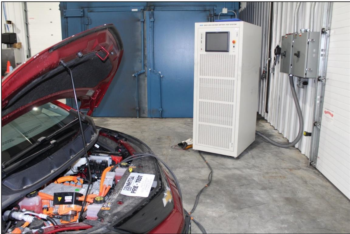
Figure 31: Over-Discharge Test Setup
