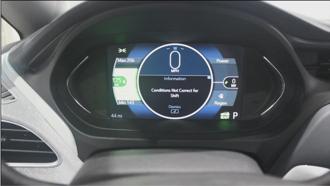
*Figure 11: Momentary Signal to Driver When Selecting Active Drive Mode Possible While External Charging Is Active.*
