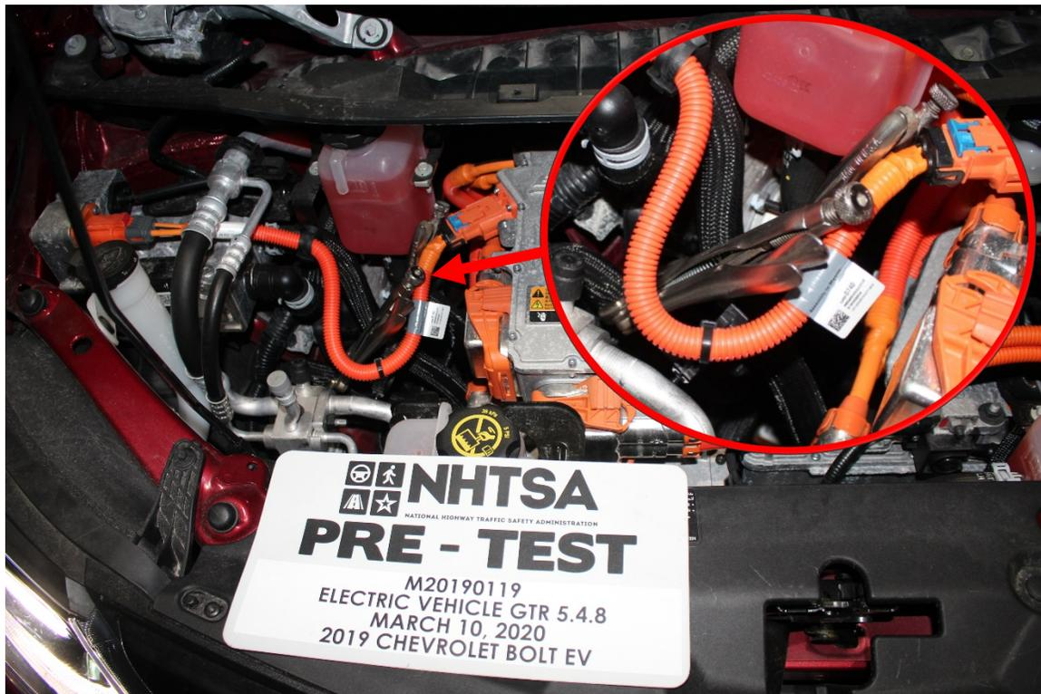
Figure 40: Over-Temperature Coolant Hose Crimps
