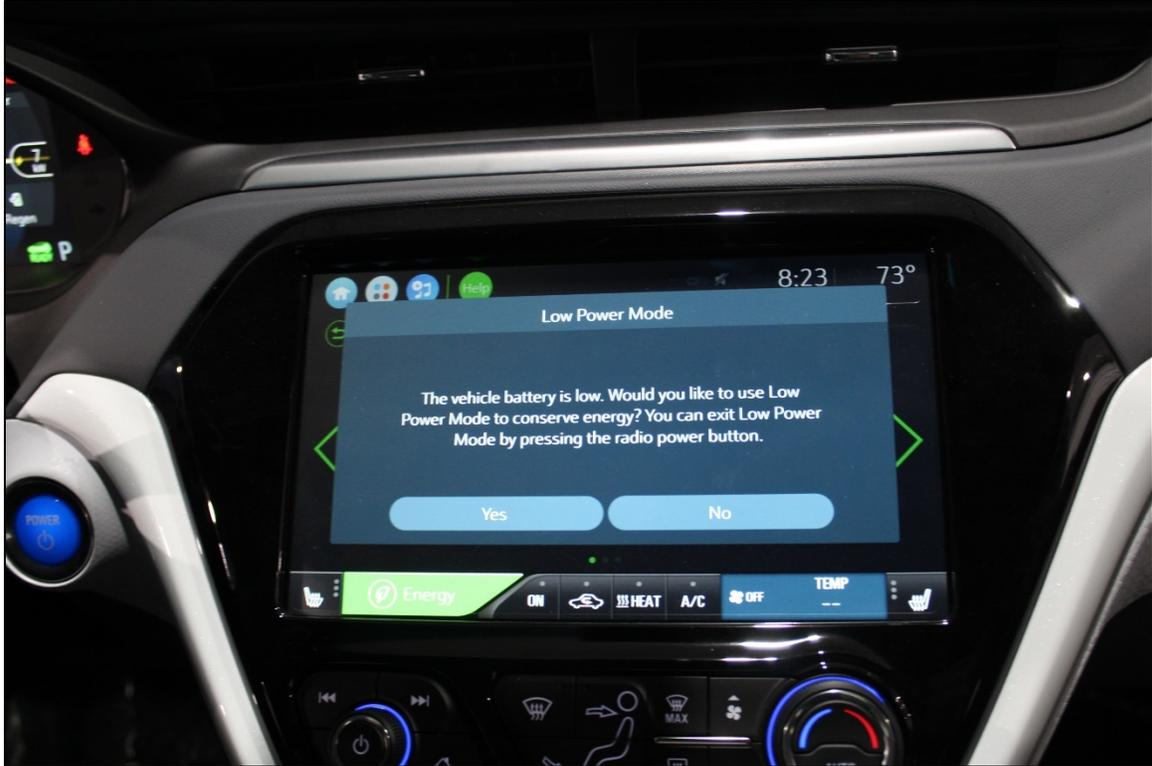
*Figure 14: Low Energy Warning on Infotainment System*
