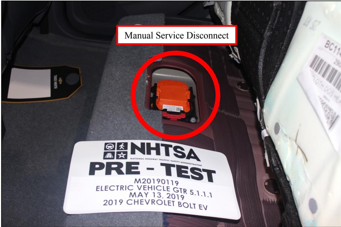
Figure 5: Vehicle Manual Service Disconnect
