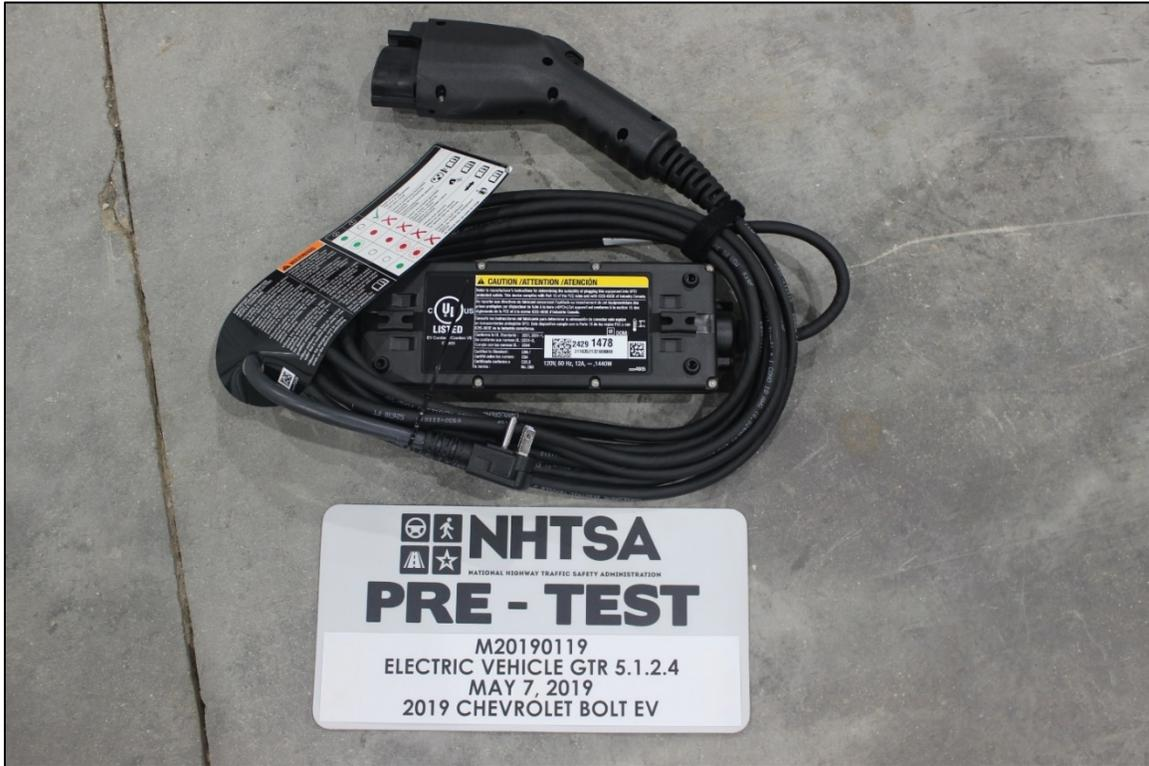
*Figure 9: Vehicle Level 1 (L1) Charger*
