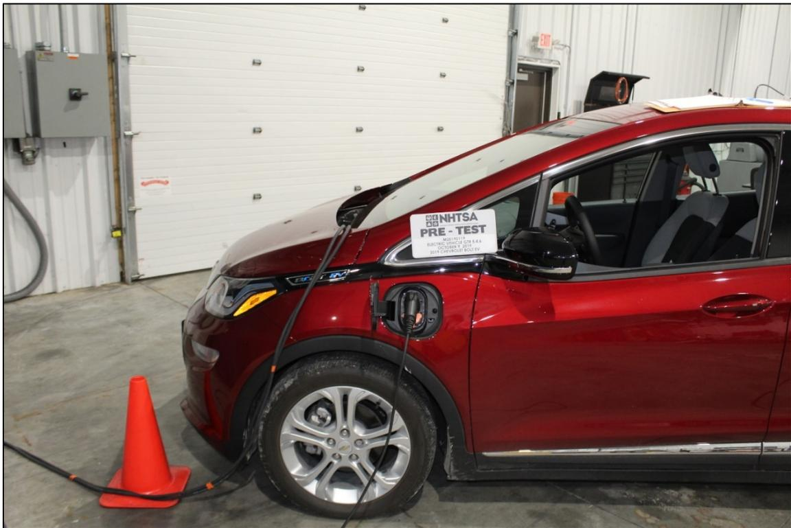
Figure 23: Over-Charge Test Setup
