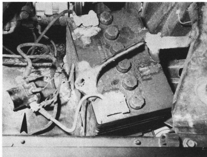
Figure 3-93. 1967 Ford LTD Relay Proximity to Battery
