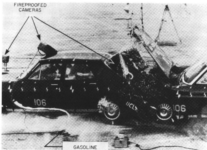
Figure 6-1. Gasoline Spray after Impact
