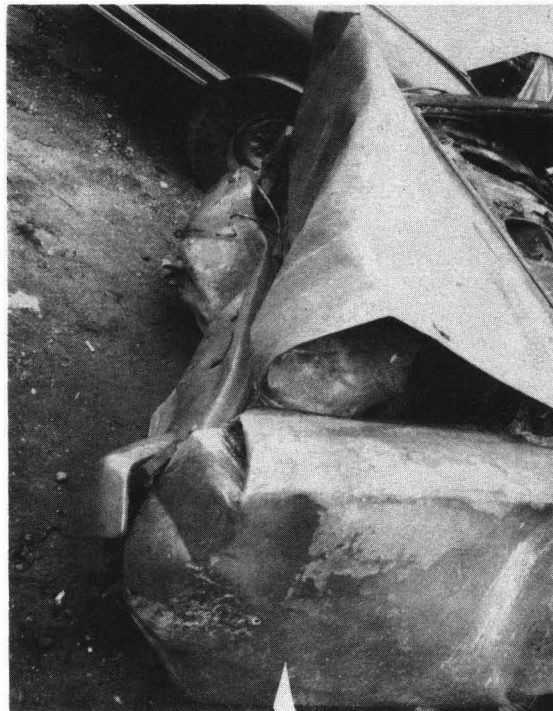
Figure 6-12. Side View of Mercury Showing Extent of Rear Deformation
