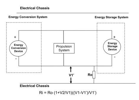
Figure 4. Measurement for V1' Voltage Across Resistor between Negative Side of the High
