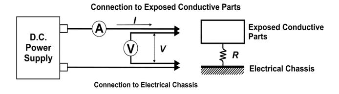
Figure 8. Connection to Determine Resistance between Exposed Conductive Parts of Electrical
