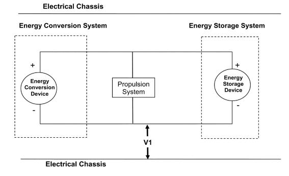
Figure 2. Measurement for V1 Voltage between the Negative Side of the High Voltage Source
