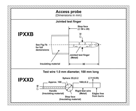
Figure 7a. Access Probes for the Tests of Direct Contact Protection. Access Probe IPXXB (top)
