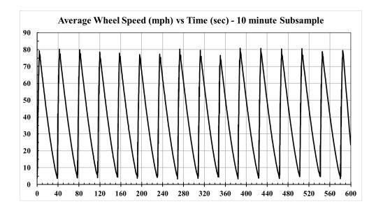
Figure 3 - Drive profile on dynamometer to quickly raise the temperature of the REESS. (For
