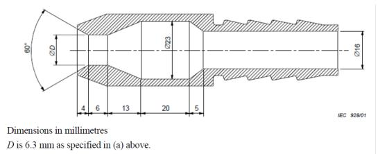
Figure 9. Standard Nozzle for IPX5 Water Exposure Test
