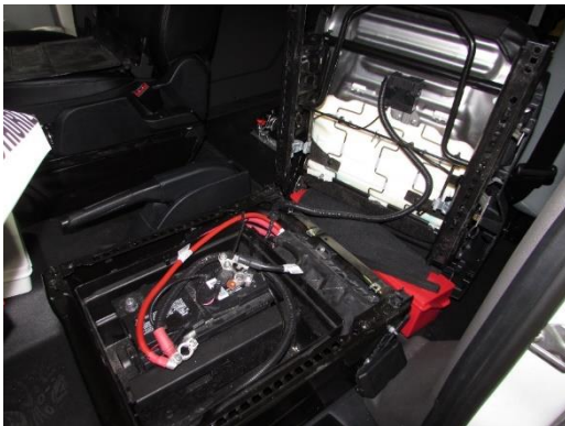
Battery located under driver's seat
