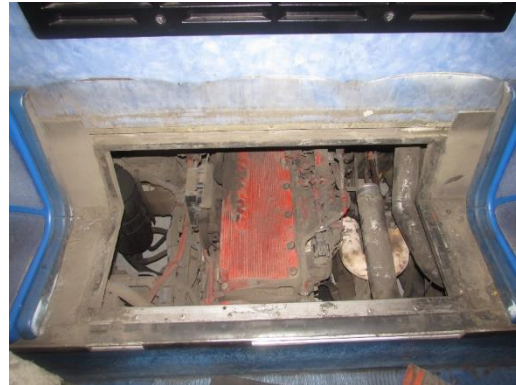
Back seat access panel to engine block
