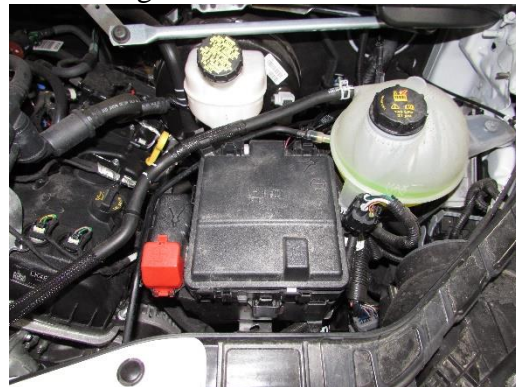
Battery cable terminal in engine compartment
