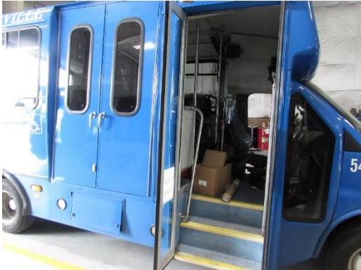
Overall view with battery compartment under wheelchair access door
