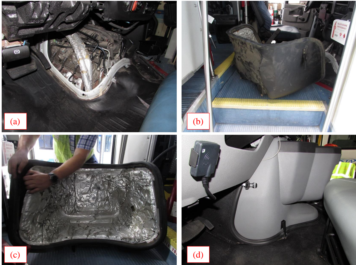
Figure 16. Pictures of engine extension and cowling in MB1 (a-c) and MB5 (d)
