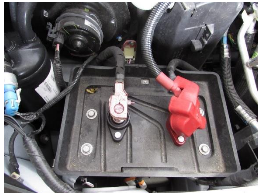
Battery distribution area in engine compartment (no battery)
