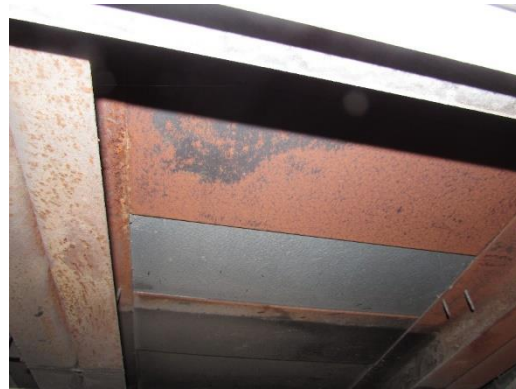
View of bus floor directly above batteries
