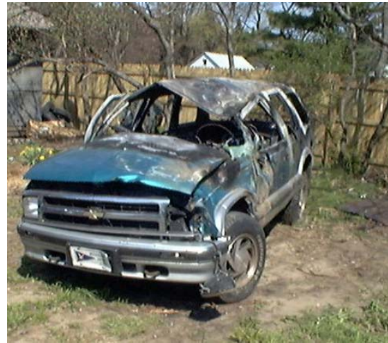
Figure 5. Major Fire after Rollover with Engine Compartment Origin – NASS Case 2001-18-58
