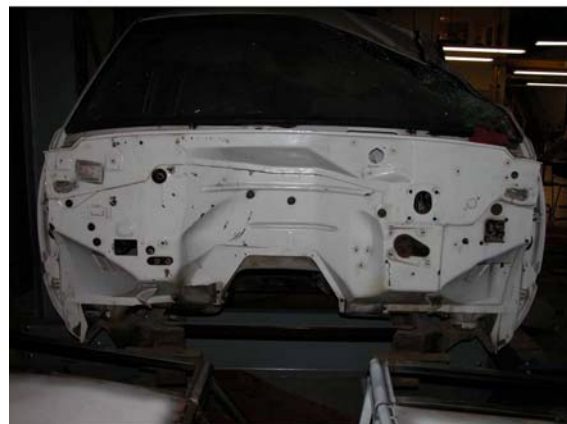
Figure 11 – Vehicle Firewall with Small Openings
