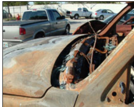
Figure 12 – Vehicle with Plastic Cowl Consumed
