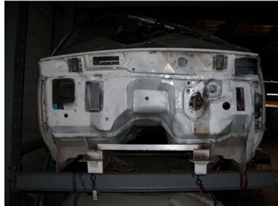
Figure 10 – Vehicle Firewall with Large Openings
