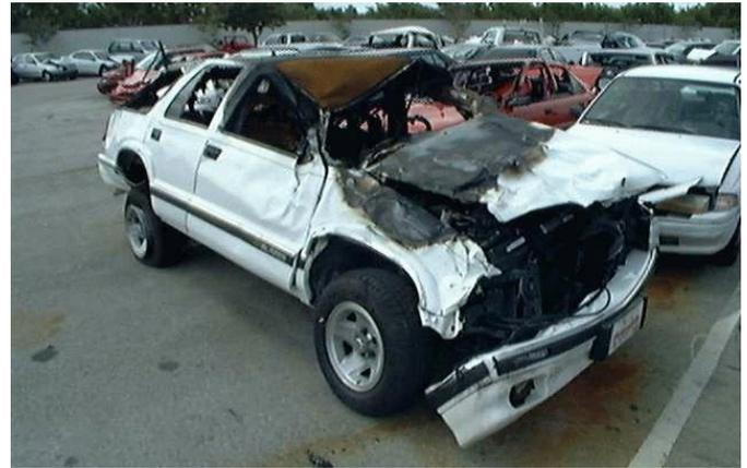
**Figure 52. Major Fire after Rollover with Engine Compartment Origin – NASS Case 1997-41-126**
