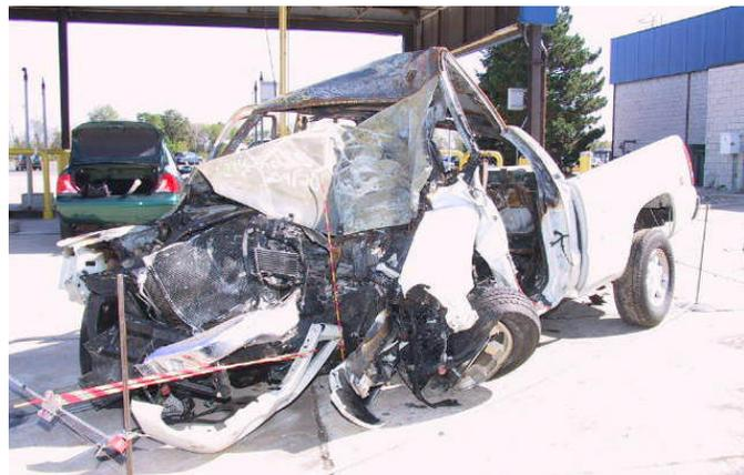
**Figure 15: Damaged Vehicle with Fire Related Fatalities – Case 2005-12-160**
