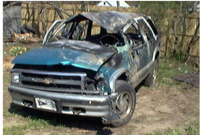
**Figure 53. Major Fire after Rollover with Engine Compartment Origin – NASS Case 2001-13-58**
