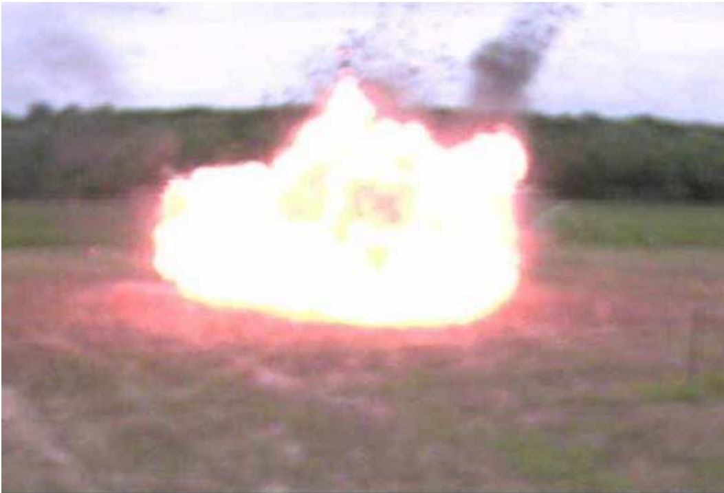
Figure 2. Hydrogen Tank Burst in FMVSS 304-Like Test
