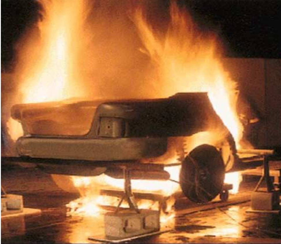
Figure 3. ECE R-34 Bonfire Test
