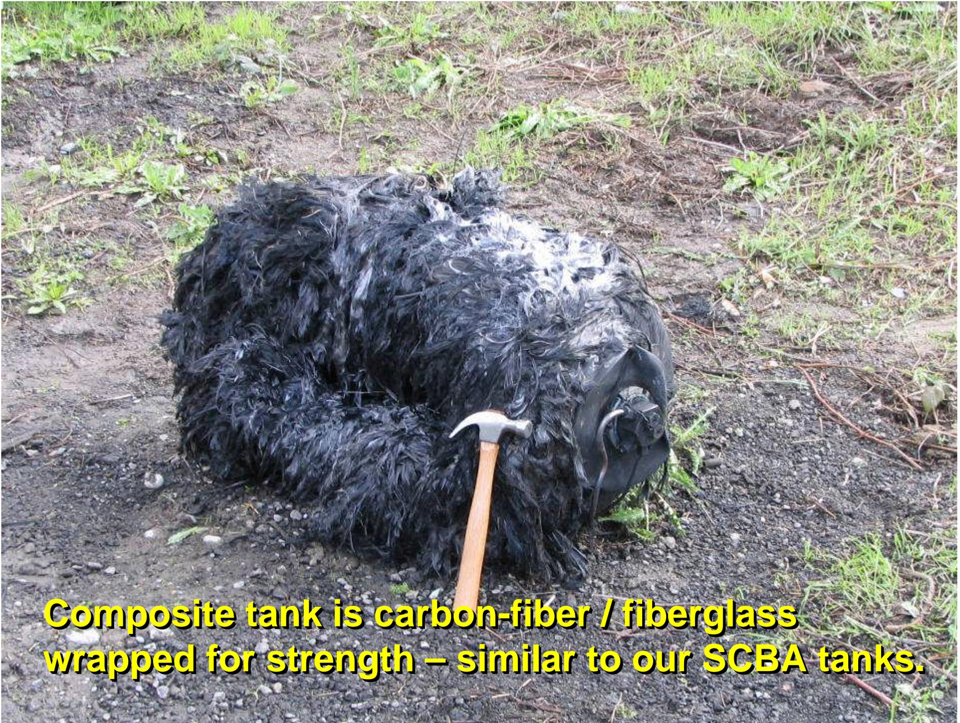
**Composite tank is carbon-fiber / fiberglass wrapped for strength – similar to our SCBA tanks.**
