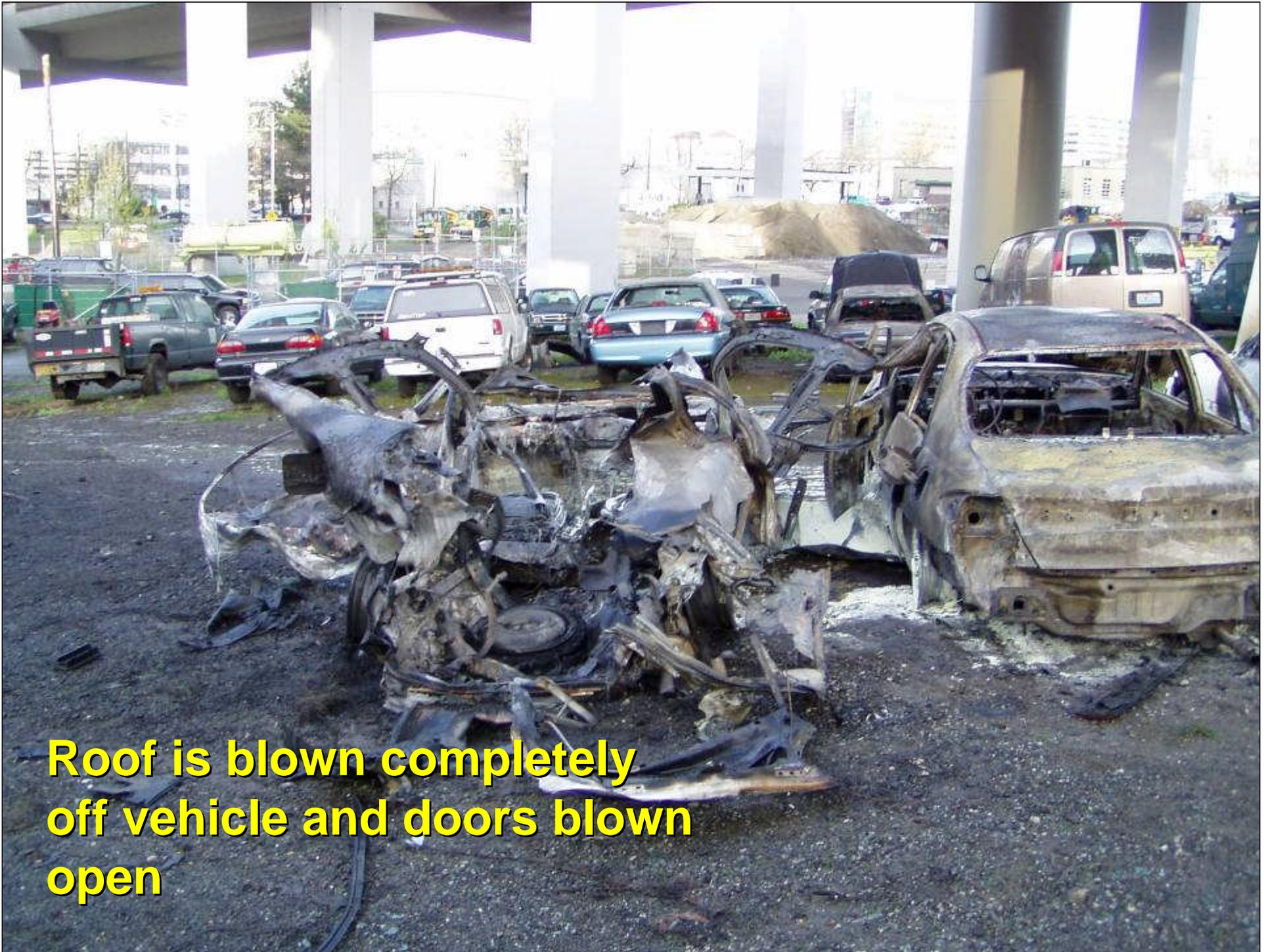
**Roof is blown completely
