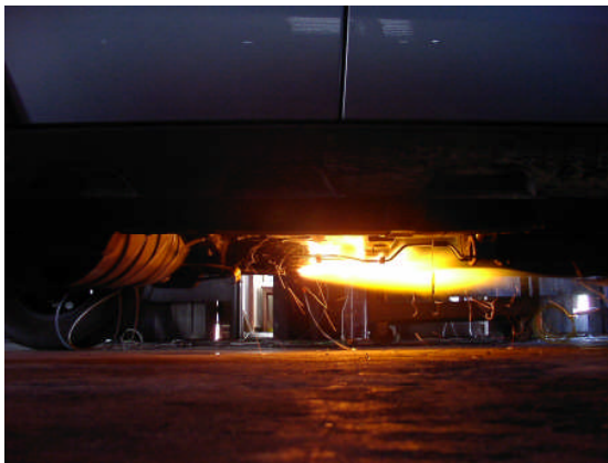
Figure 9: Leakage flame during test
