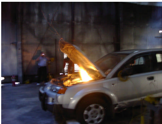
Figure 5: Fuel line leakage – hood open
