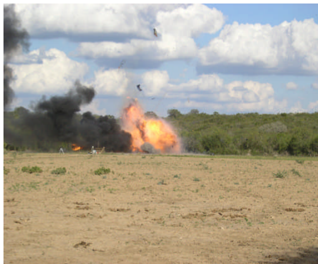
Figure 3. Fireball from tank burst
