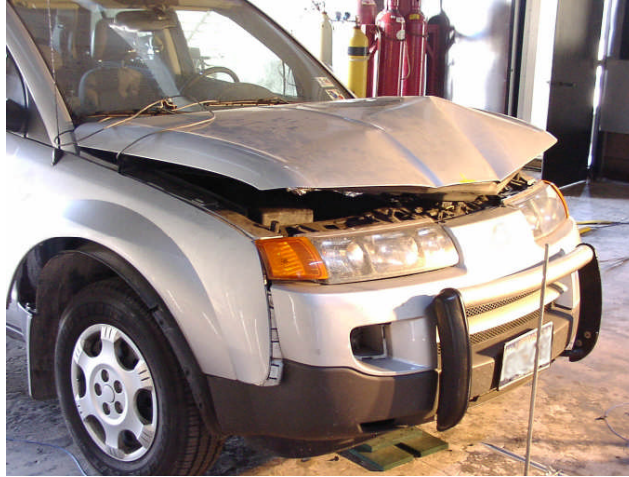
Figure 4. Damage to vehicle during series 2 leakage tests
