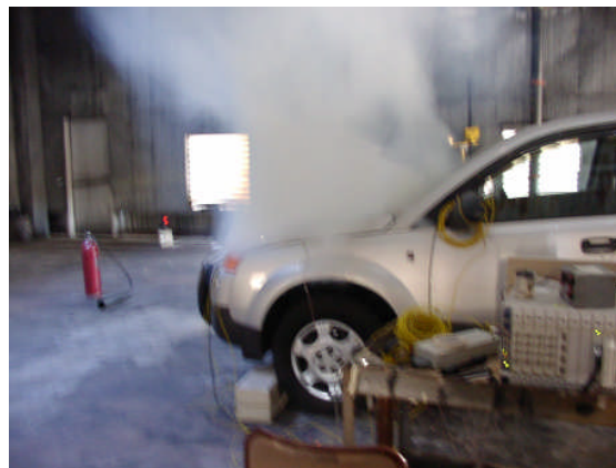
Figure 6: Fuel line leakage – hood closed
