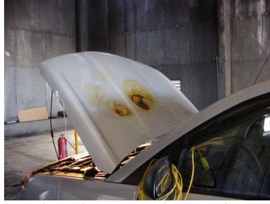
Figure 8: Hood damage - outside
