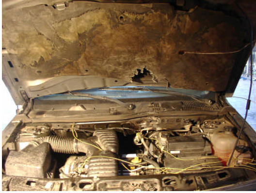
Figure 7: Hood damage – underside
