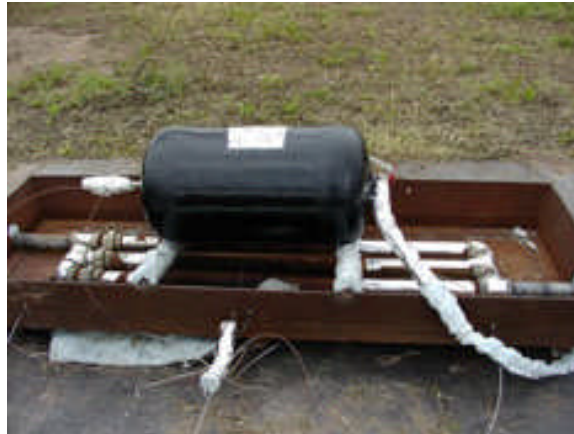
Figure 1. Hydrogen fuel tank in bonfire test fixture
