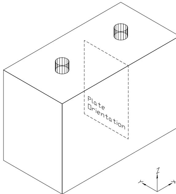
**Figure 2. Battery Axis Definition.**
