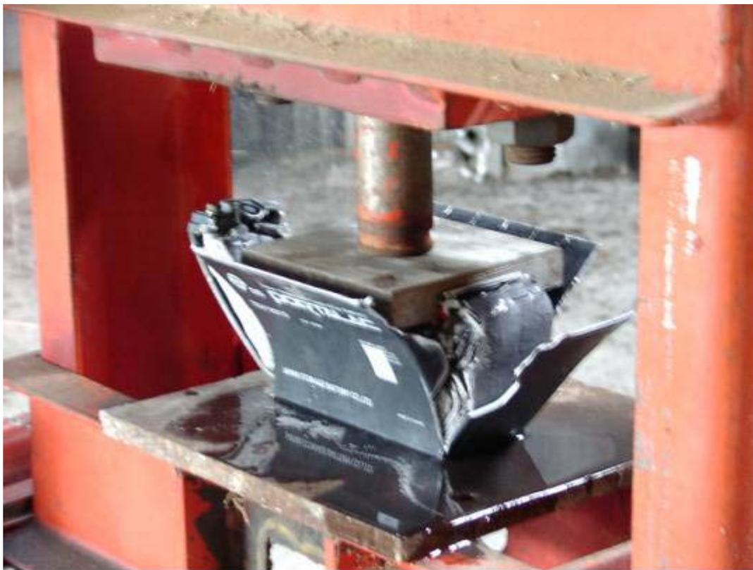
**Figure B-12. Z-Axis Crushing of 12V Battery.**
