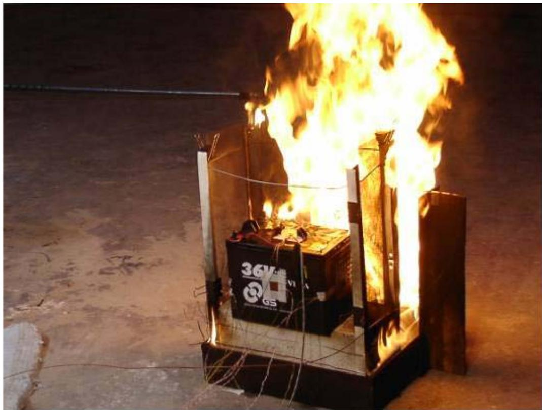
**Figure B-24. Ignition of 36V Battery During Radiant Exposure Test.**
