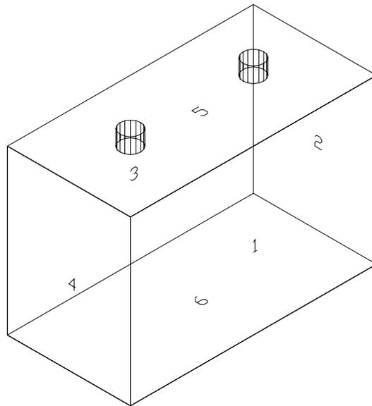
**Figure 1. Thermocouple / Heat Flux Transducer Layout.**
