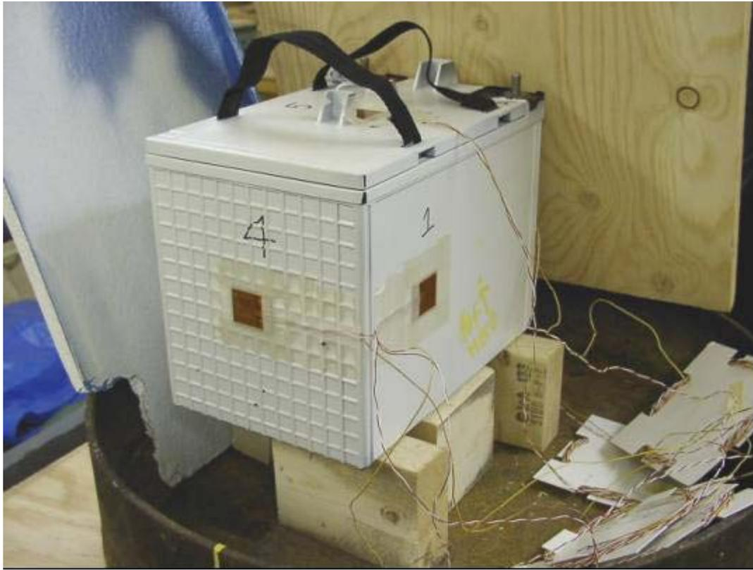
**Figure B-7. Hot Spot Indicated on 36V Battery.**
