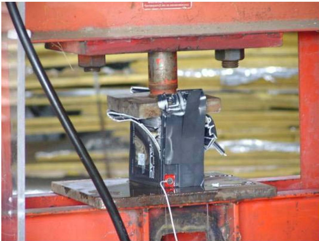
**Figure B-10. X-Axis Crushing of 12V Battery.**
