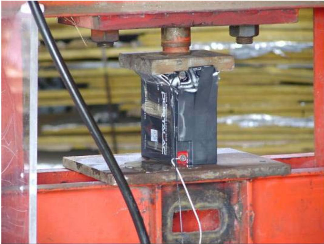
**Figure B-9. X-Axis Crushing of 12V Battery.**
