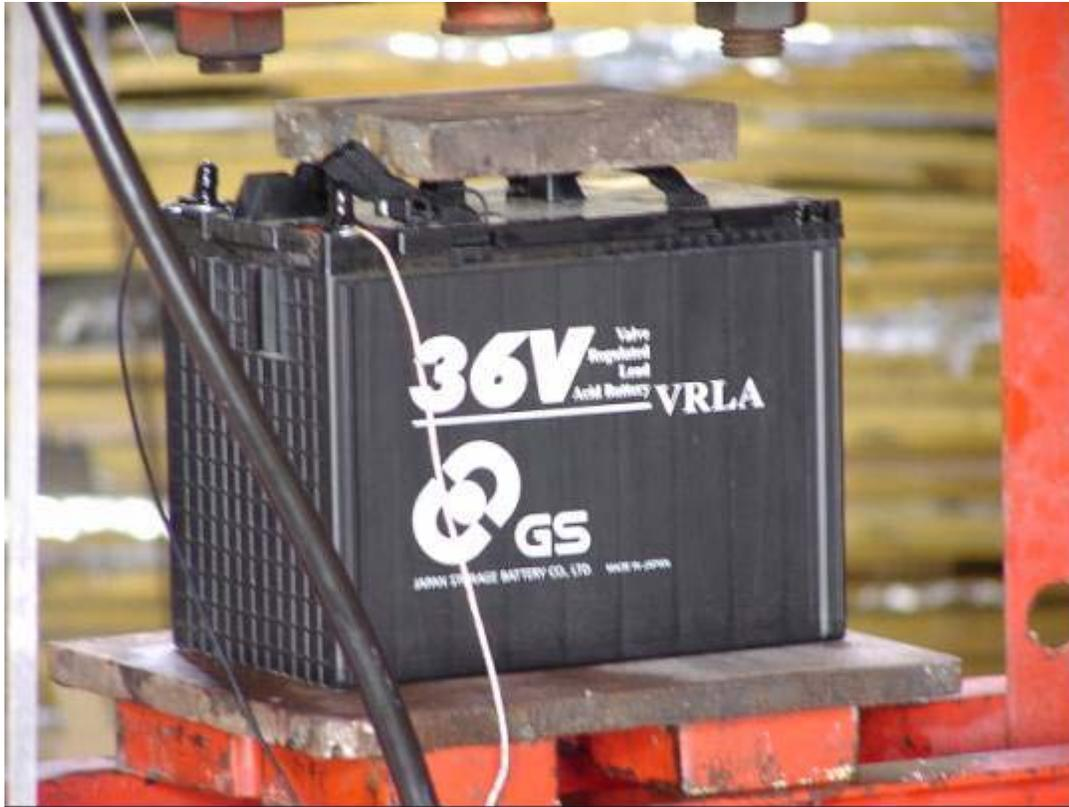
**Figure B-17. 36V Battery Prior to Z-Axis Crush Test.**
