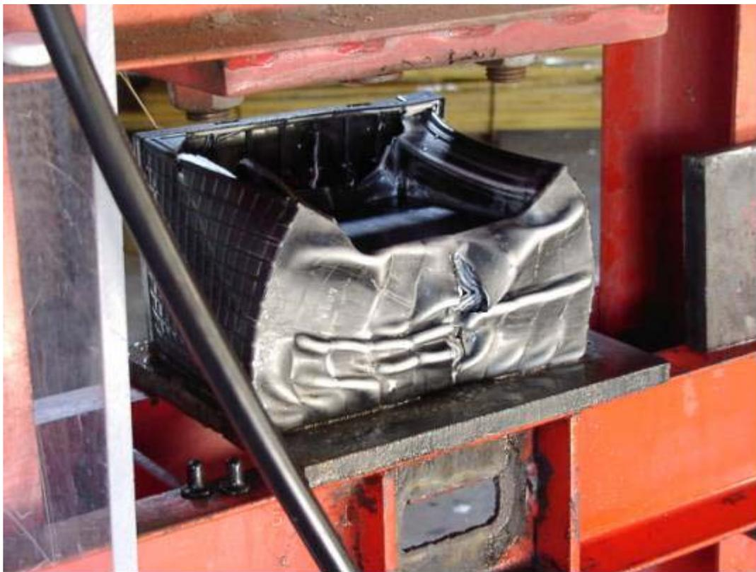
**Figure B-16. 36V Battery Following Crush Test.**
