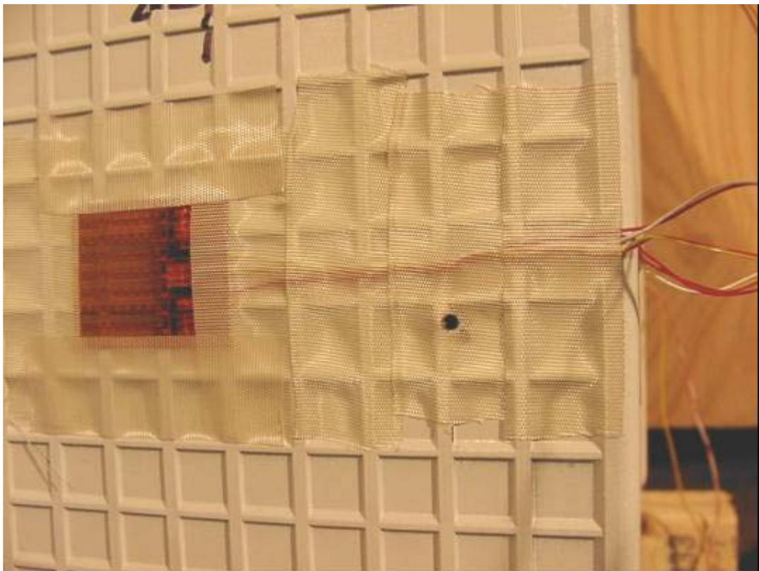
**Figure B-6. Penetration Hole Through 36V Battery (Test No. 1).**
