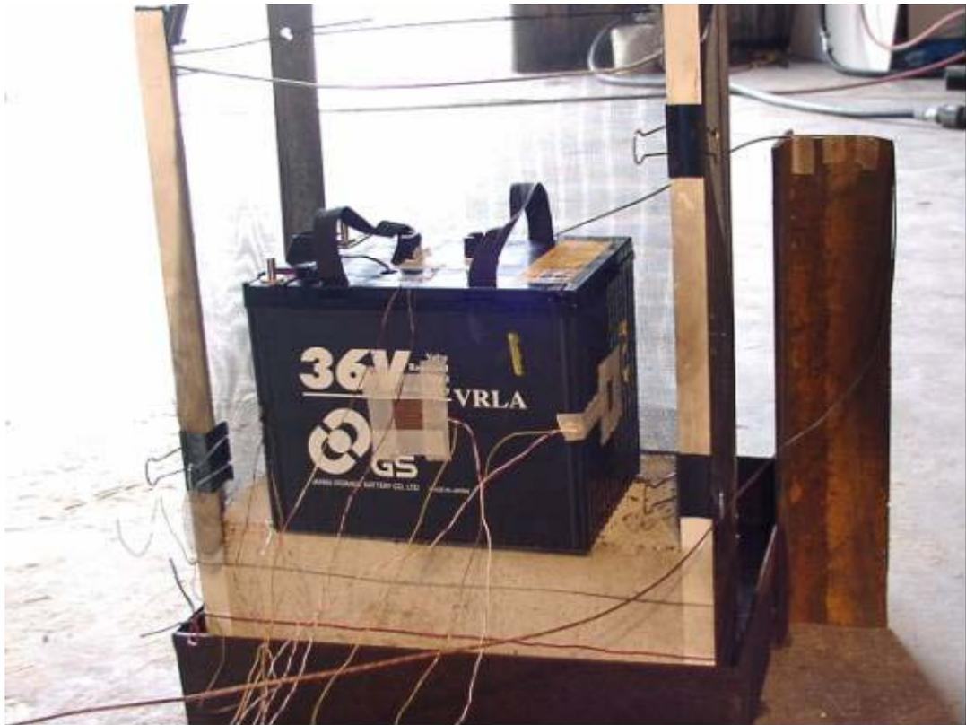
**Figure B-22. 36V Battery prior to Radiant Exposure Test.**
