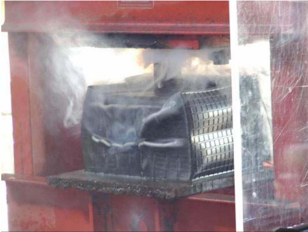
**Figure B-15. Sulfuric Acid Vapors Emitting from 36V Battery During Y-Axis Crush Test No. 1.**
