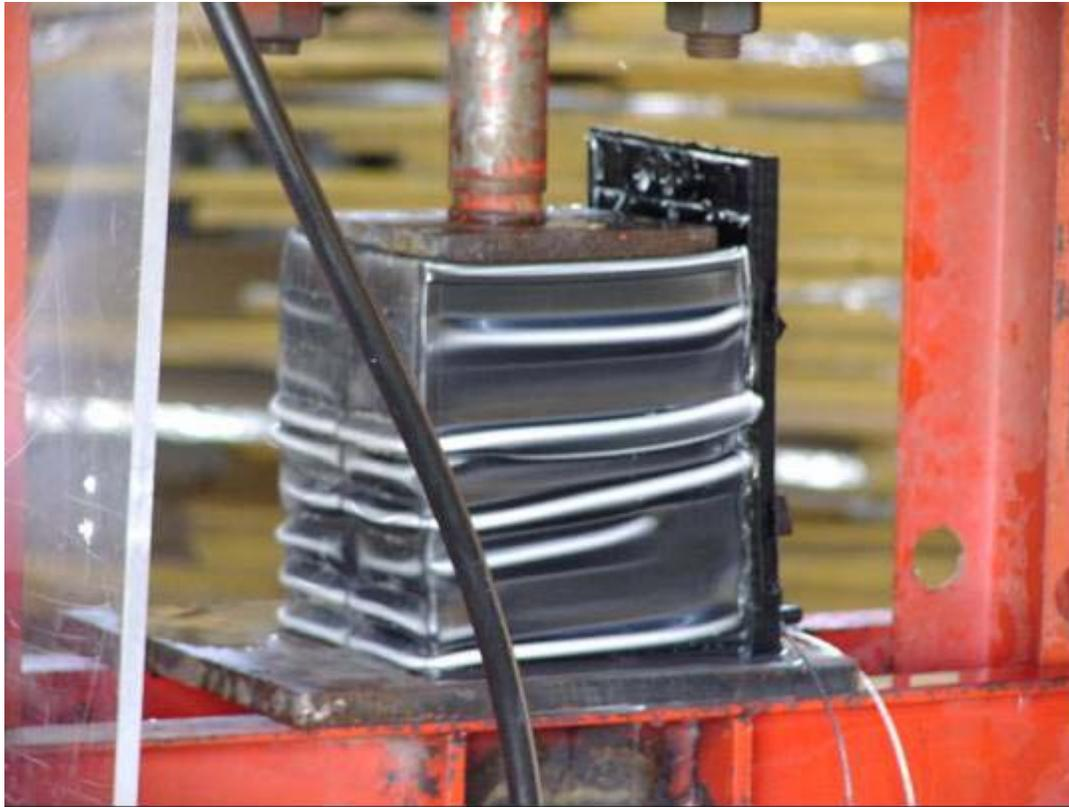
**Figure B-13. Z-Axis Crushing of 36V Battery.**
