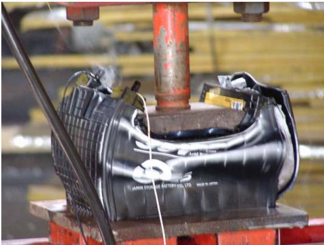
**Figure B-18. 36V Battery During Z-Axis Crush. Note Arcing to Crush Plate.**
