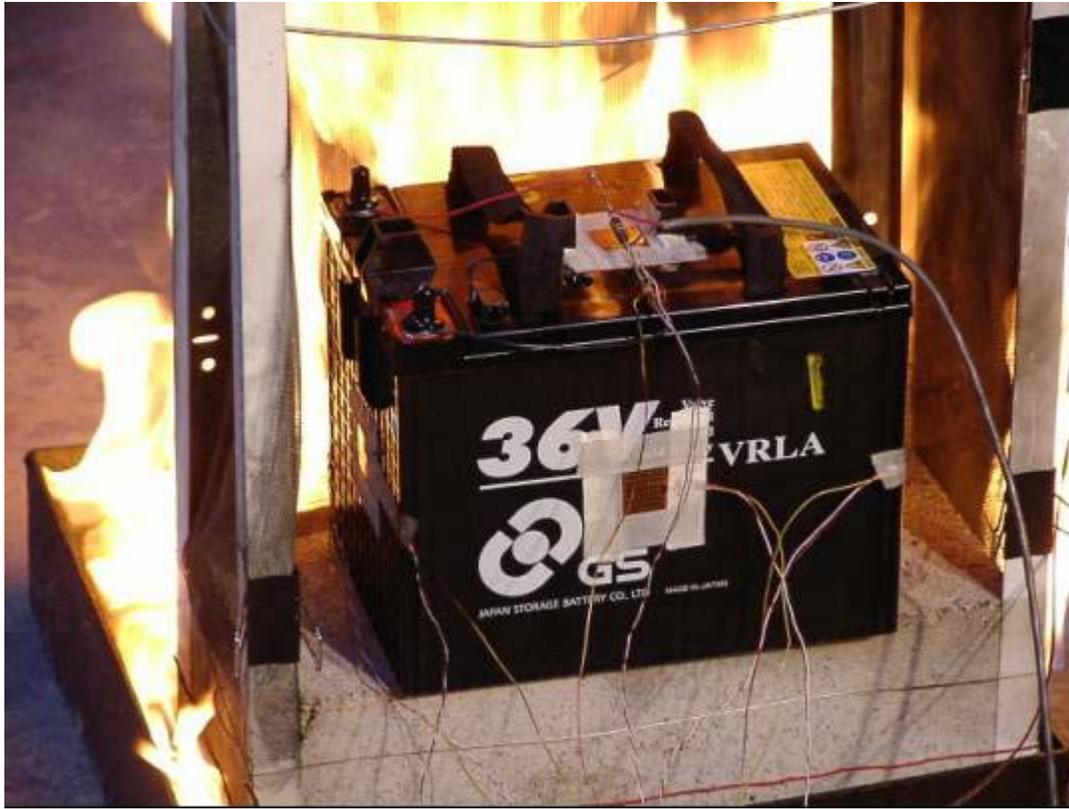
**Figure B-23. 36V Battery at Beginning of Radiant Exposure Test.**
