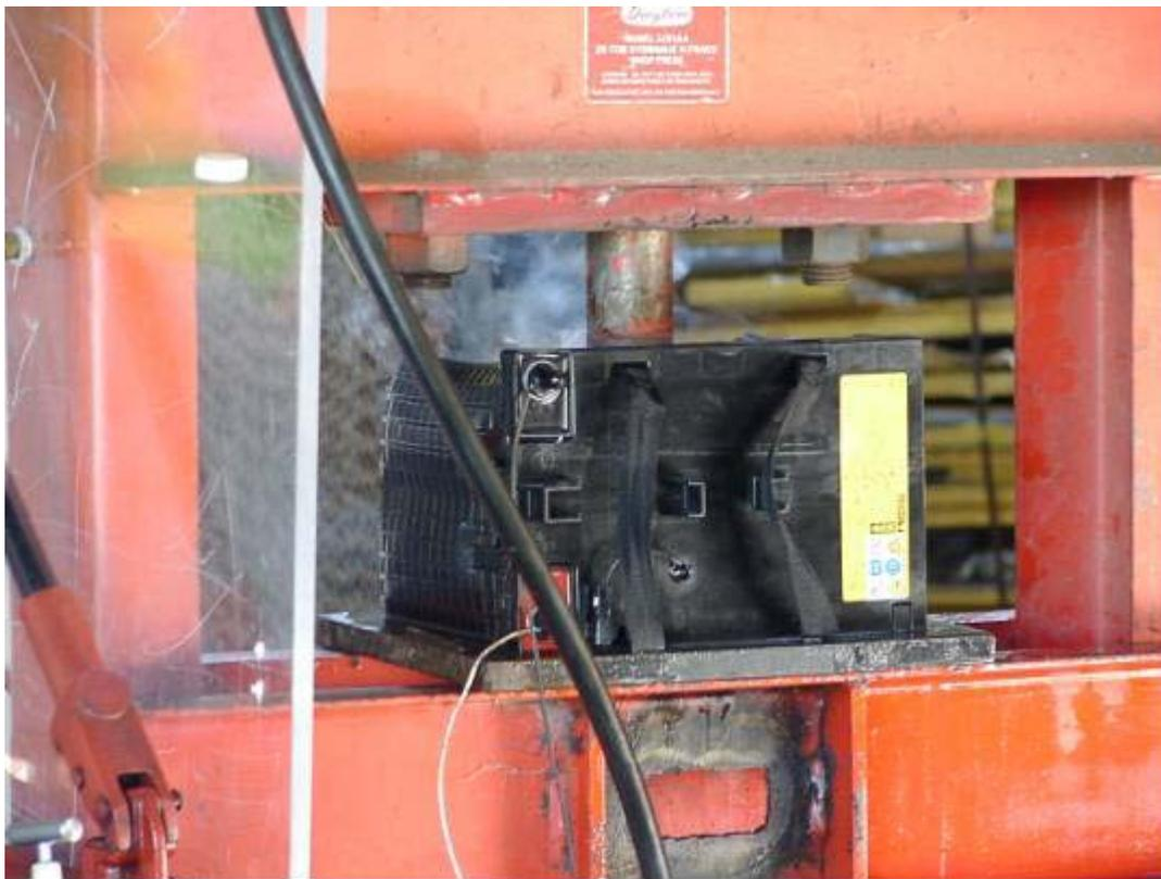
**Figure B-14. Y-Axis Crushing of 36V Battery.**
