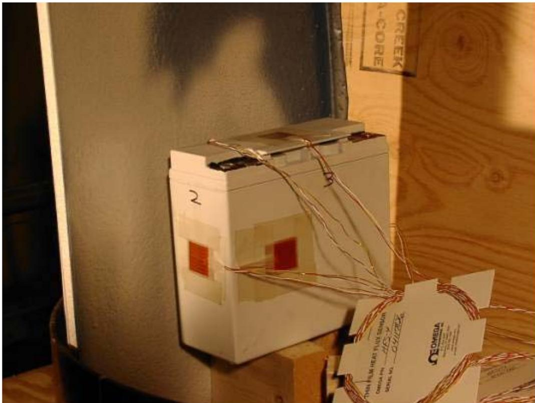
**Figure B-2. 12V Battery prior to Penetration Test.**
