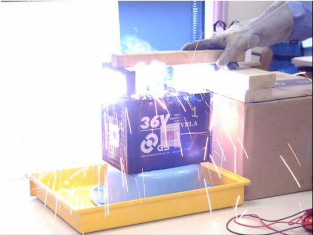
**Figure B-29. Application of Hard Short to 36V Battery.**
