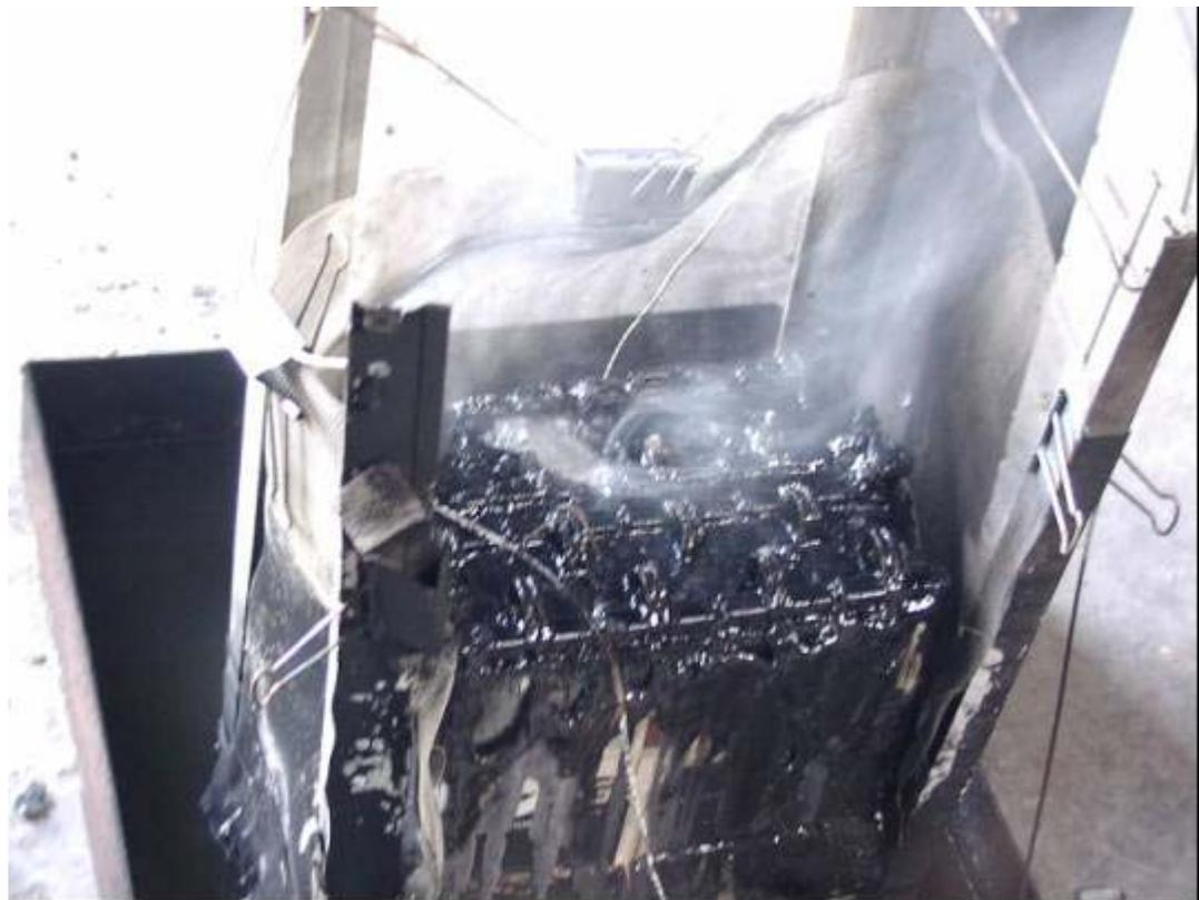
**Figure B-26. 36V Battery Following Radiant Exposure Test No. 2.**
