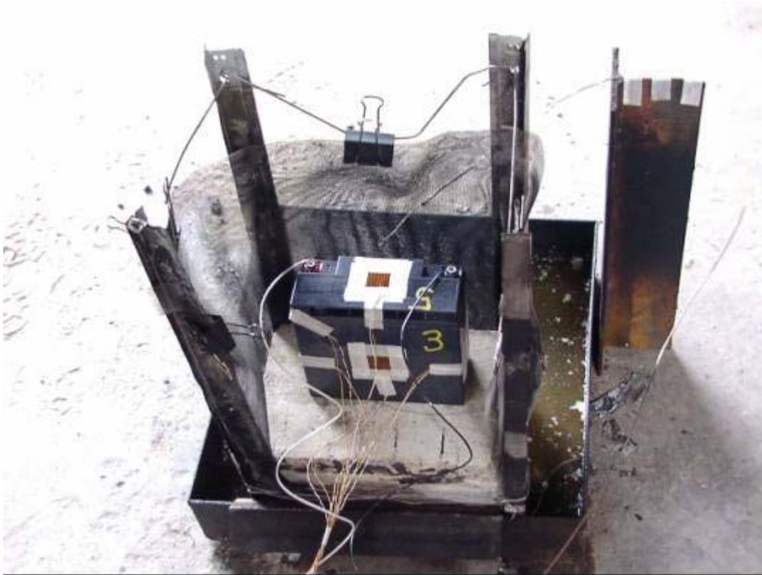
**Figure B-19. 12V Battery Prior to Radiant Exposure Test.**
