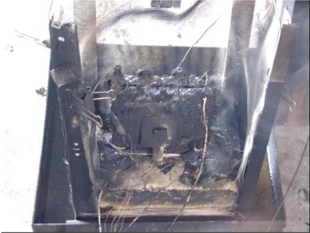
**Figure B-21. 12V Battery Following Radiant Exposure Test.**
