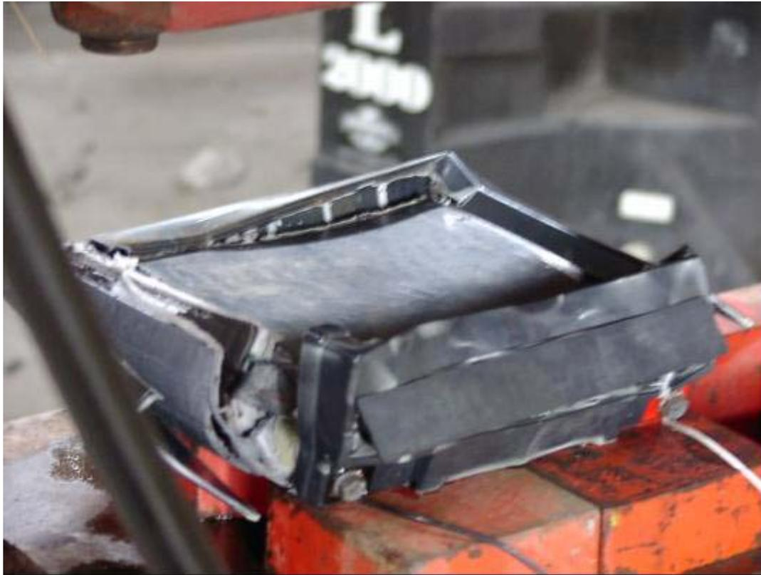
**Figure B-11. 12V Battery Following Y-Axis Crushing.**
