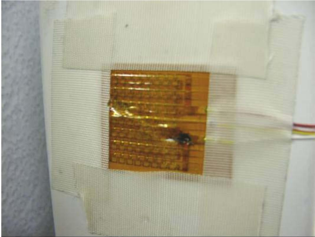
**Figure B-3. Penetration Hole in 12V Battery (Through Heat Flux Sensor).**
