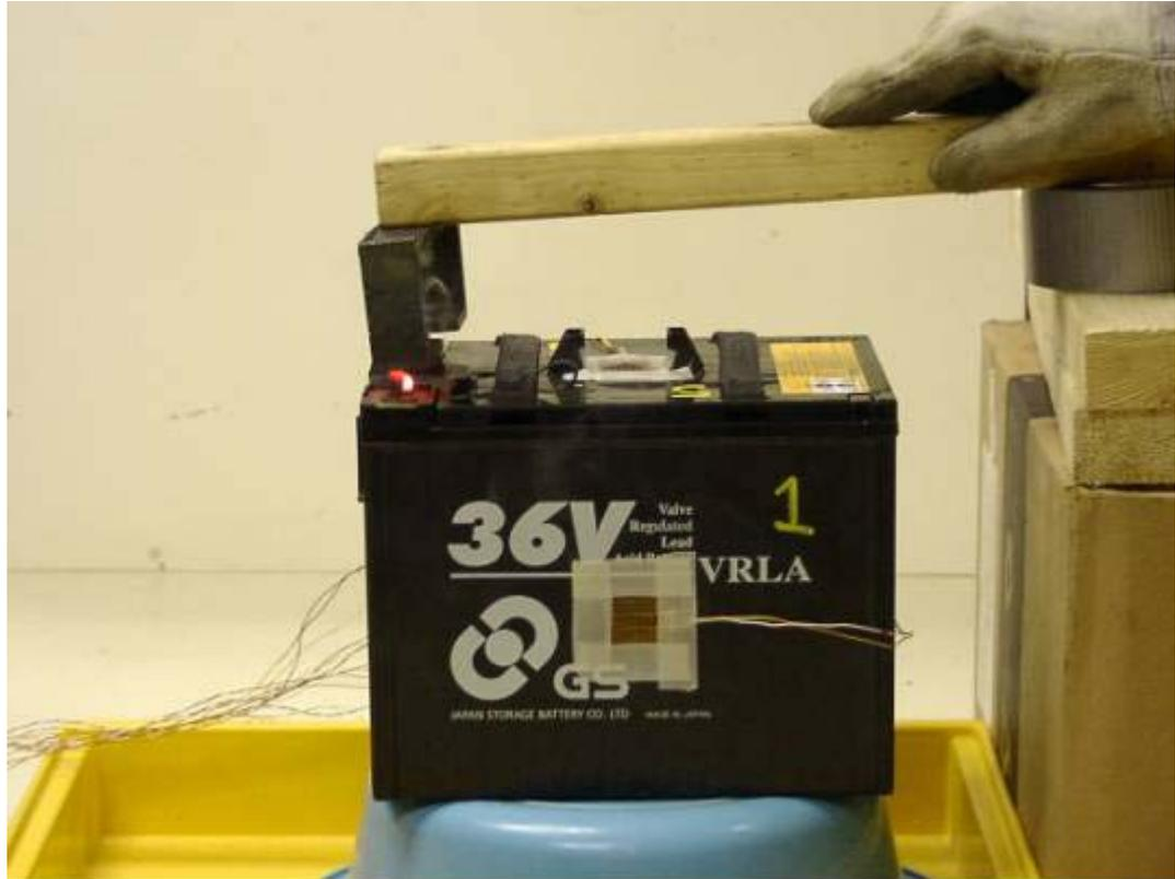
**Figure B-30. Red-Hot Peg Shown after Application of Hard Short to 36V Battery.**
