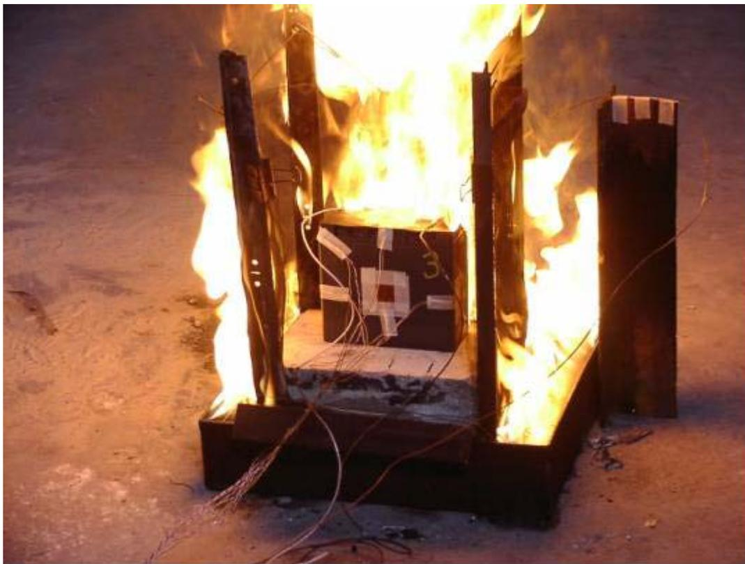
**Figure B-20. 12V Battery Immediately after Ignition During Radiant Exposure Test.**
