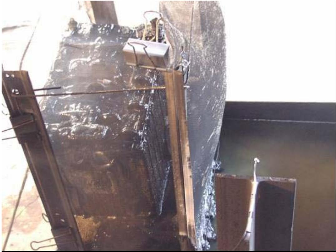
**Figure B-25. 36V Battery Following Radiant Exposure Test No. 1.**
