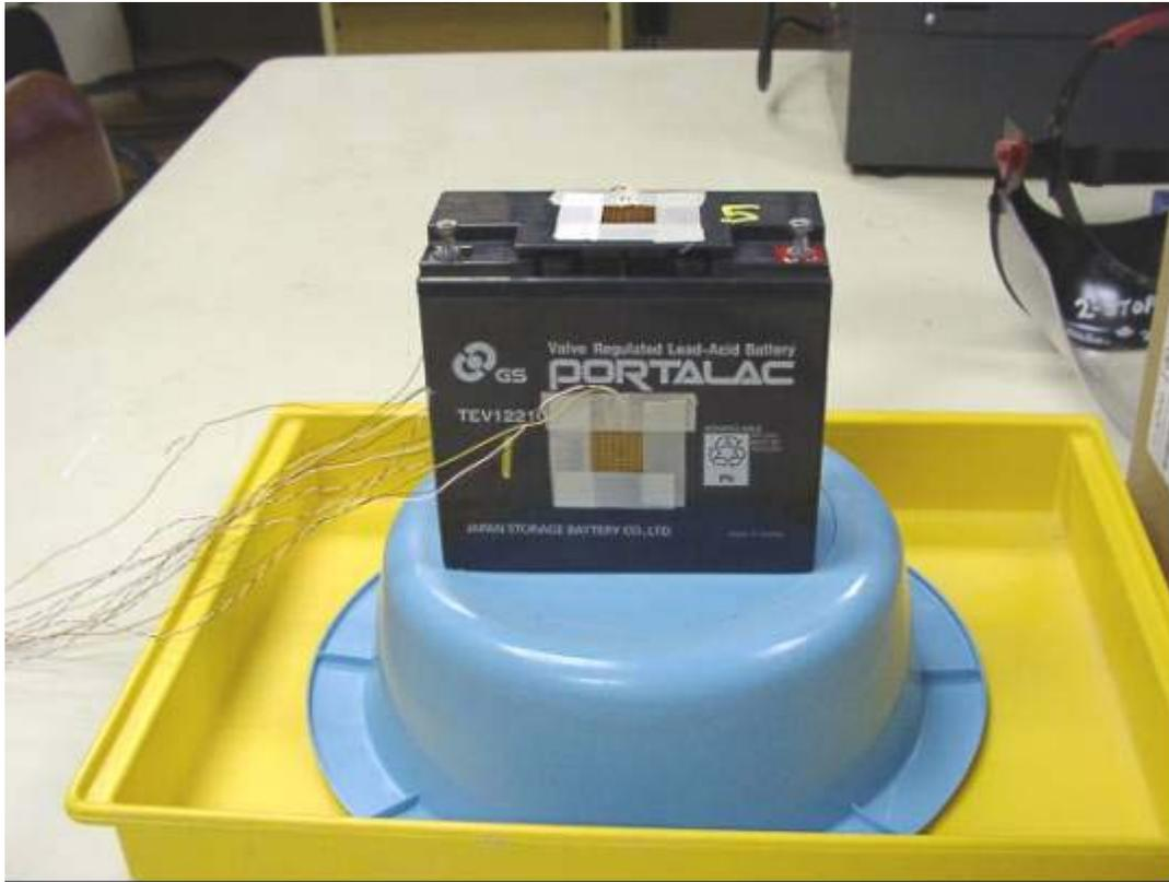
**Figure B-27. 12V Battery prior to Short Circuit Test.**
