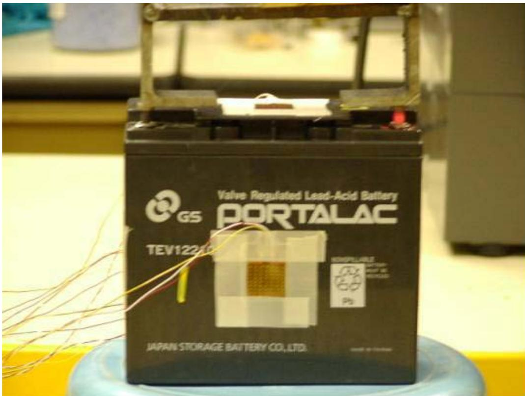
**Figure B-28. 12V Battery after Application of Hard Short (Note Red-Hot Stem).**
