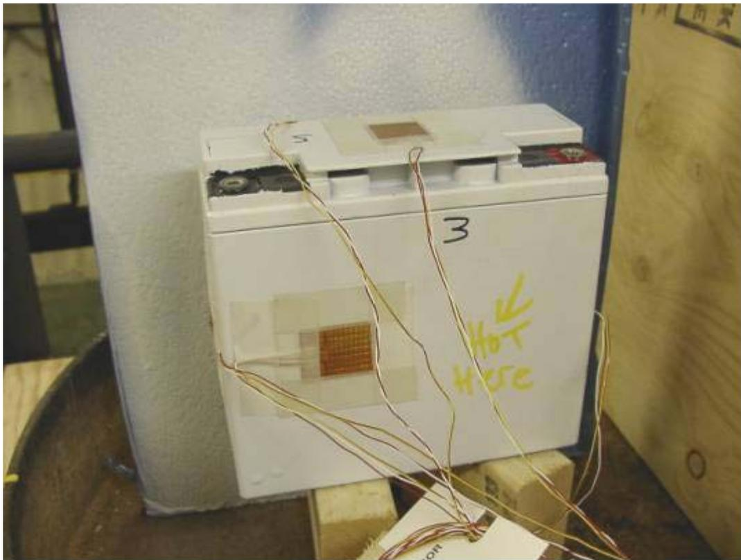
**Figure B-4. Hot Spot Indicated on 12 V Battery Following Test.**
