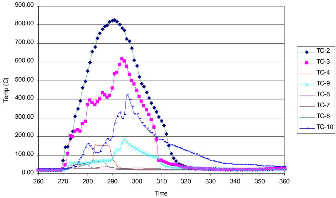
Figure 57: Thermocouple Data for Test #3 – Suppression Test on Chrysler.
