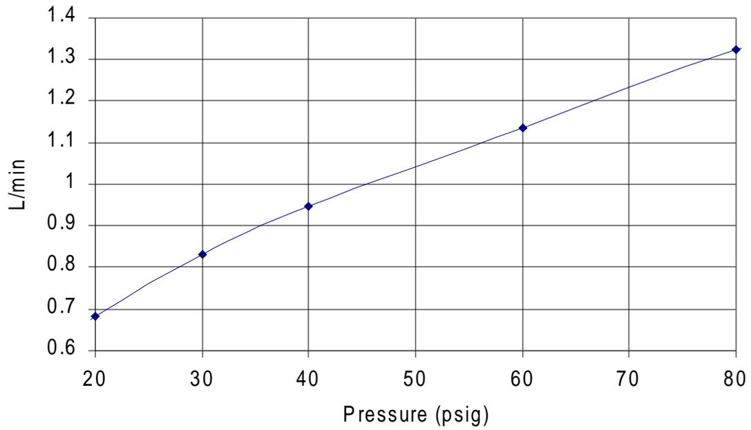
Figure 35: Solution Flow versus Pressure for BETE WL ¼ Spray Nozzle
