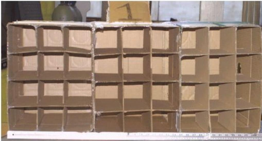
Figure 16: Box Set-Up #1: 11 cm<sup>2</sup> Channel Size
