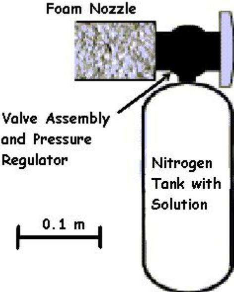
Figure 67: Integrated System Sketch of Possible Configuration of Working Foam Generator System
