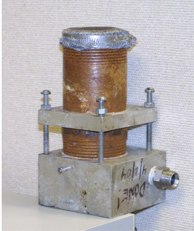
Figure 33: Foam Nozzle with Clamping Device Added to Prevent Gas Leakage
