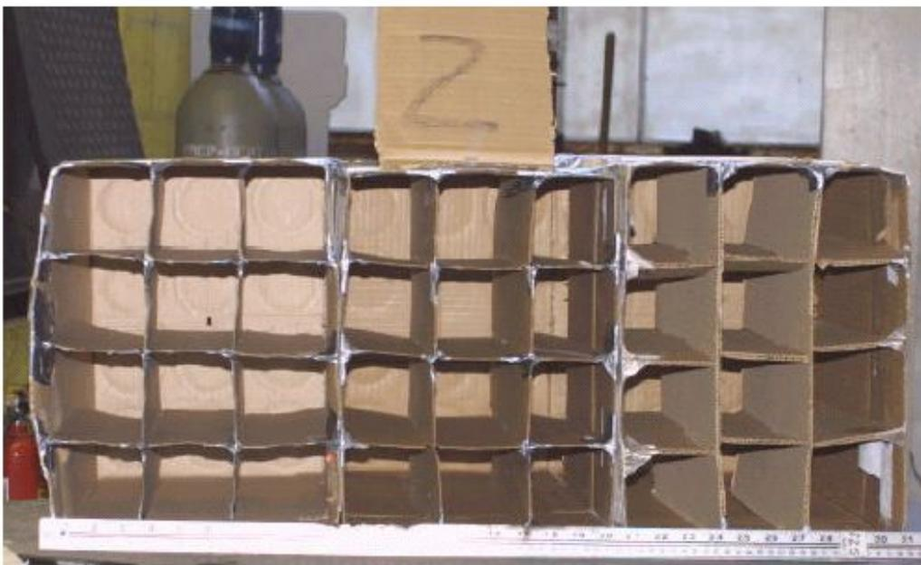
Figure 17: Box Set-Up #2: 8 cm<sup>2</sup> Channel Size
