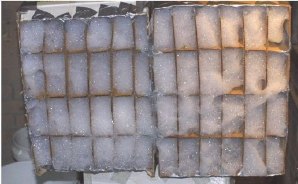
Figure 21: Box Set-Up #3 w/ 200 Expansion Ratio Foam
