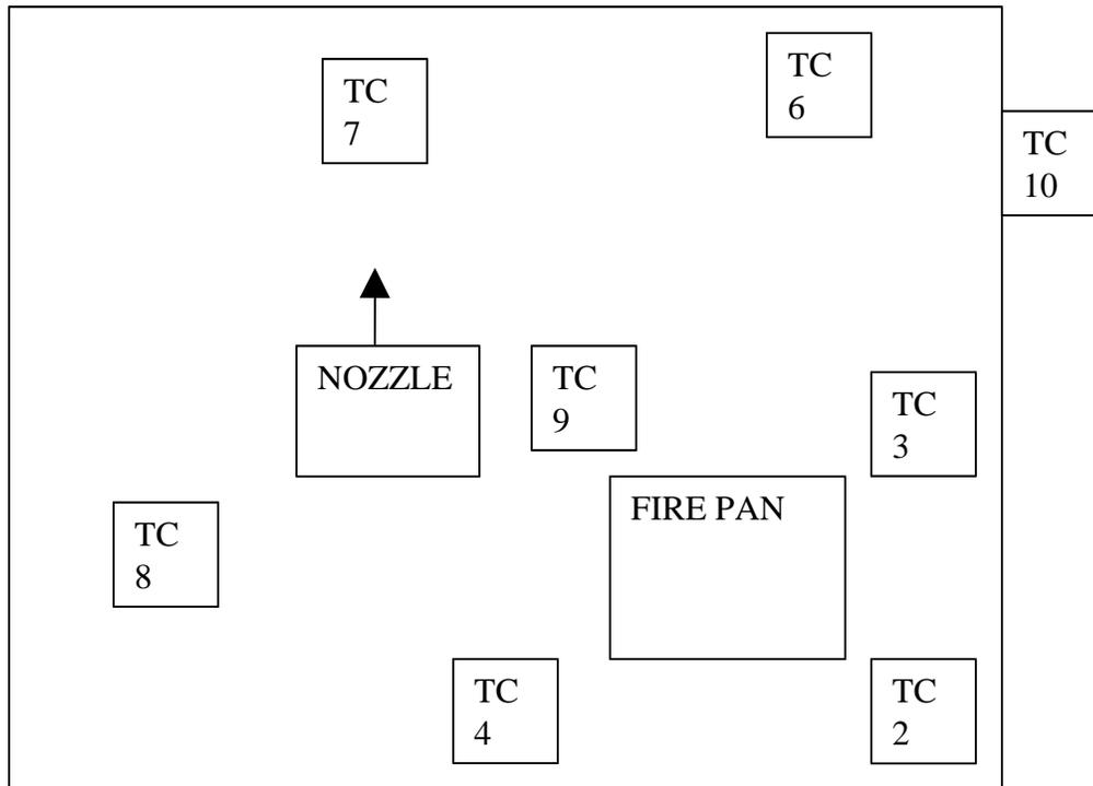
Figure 53: Arrangement of Thermocouples in Chrysler for Test #3.
