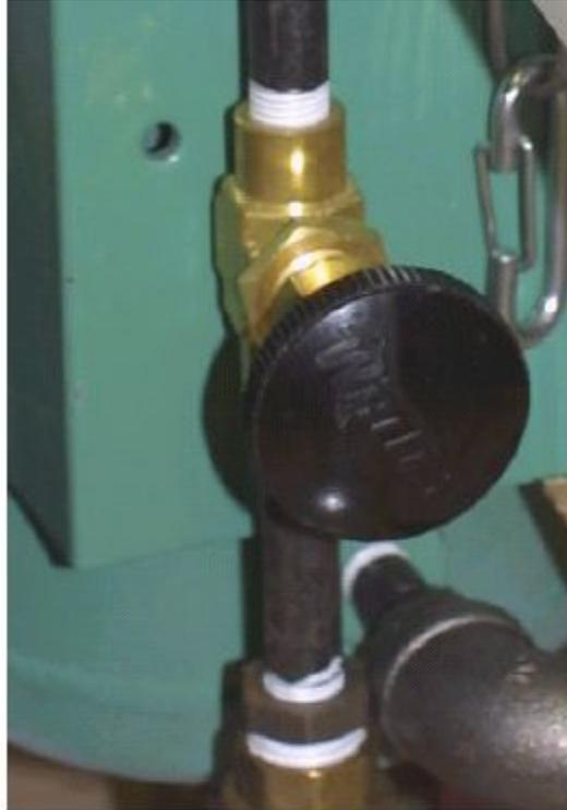
Figure 9: Needle Flow Valve (Whitey; BORF2)
