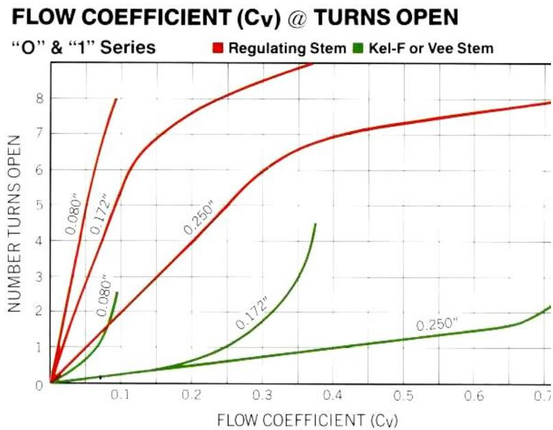
Figure 10: Cv chart for Needle Flow Valve
