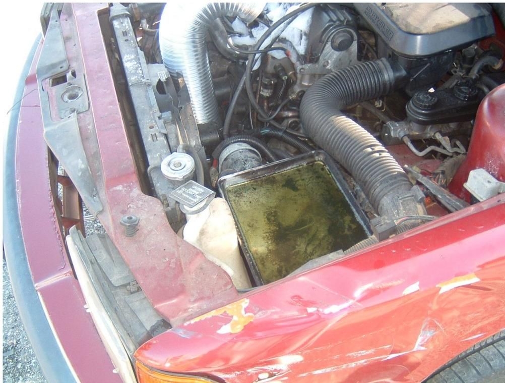
Figure 48: Position of Fuel Pan in Engine Compartment of Chrysler
