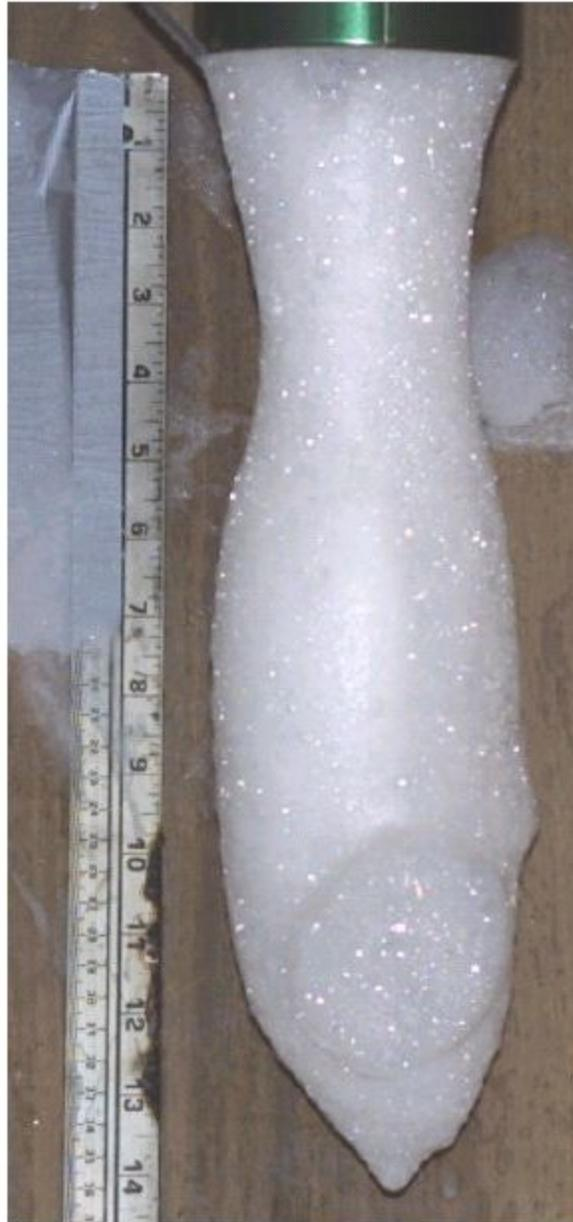
Figure 22: Foam Hang Test #1: Expansion Ratio = 220, Diameter of Pipe = 0.1 m
