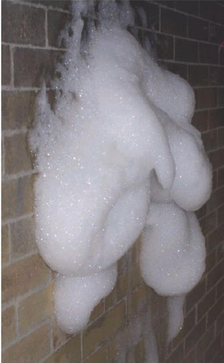
Figure 24: Foam Hanging From Wall: Expansion Ratio = 220
