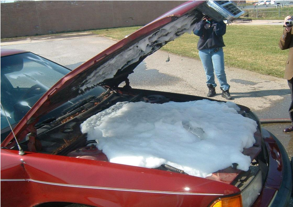
Figure 52: Foam Filled Engine Compartment of Chrysler (Side View)
