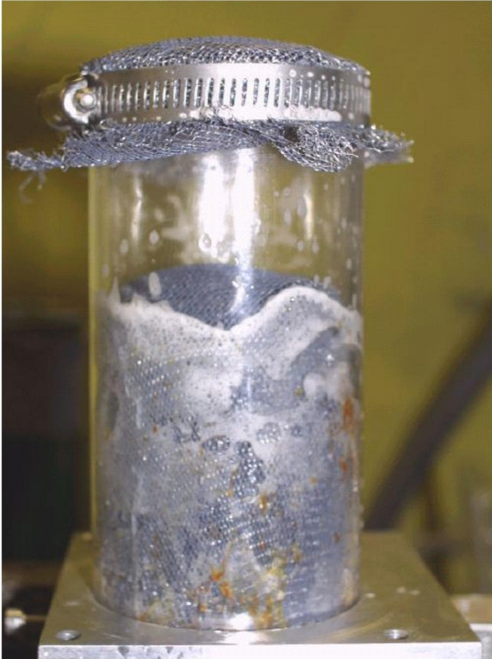
Figure 11: Side View of Mesh Configuration in Nozzle Pipe
