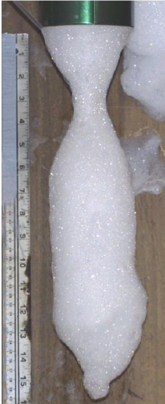
Figure 23: Foam Hang Test #2: Expansion Ratio = 220, Diameter of Pipe = 0.1 m
