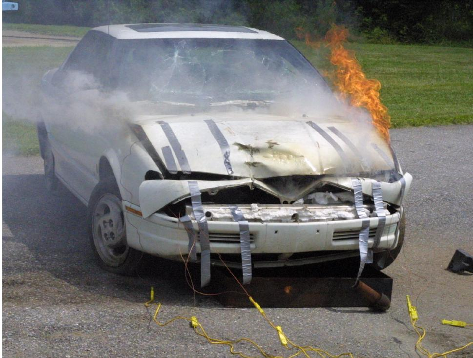
Figure 45: Saturn During Un-Suppressed Burn
