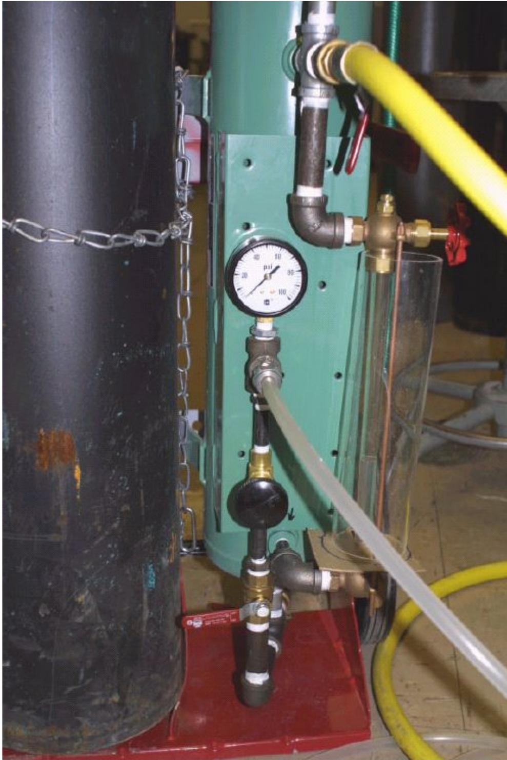
Figure 6: Solution Tank, Level Gauge and Connections
