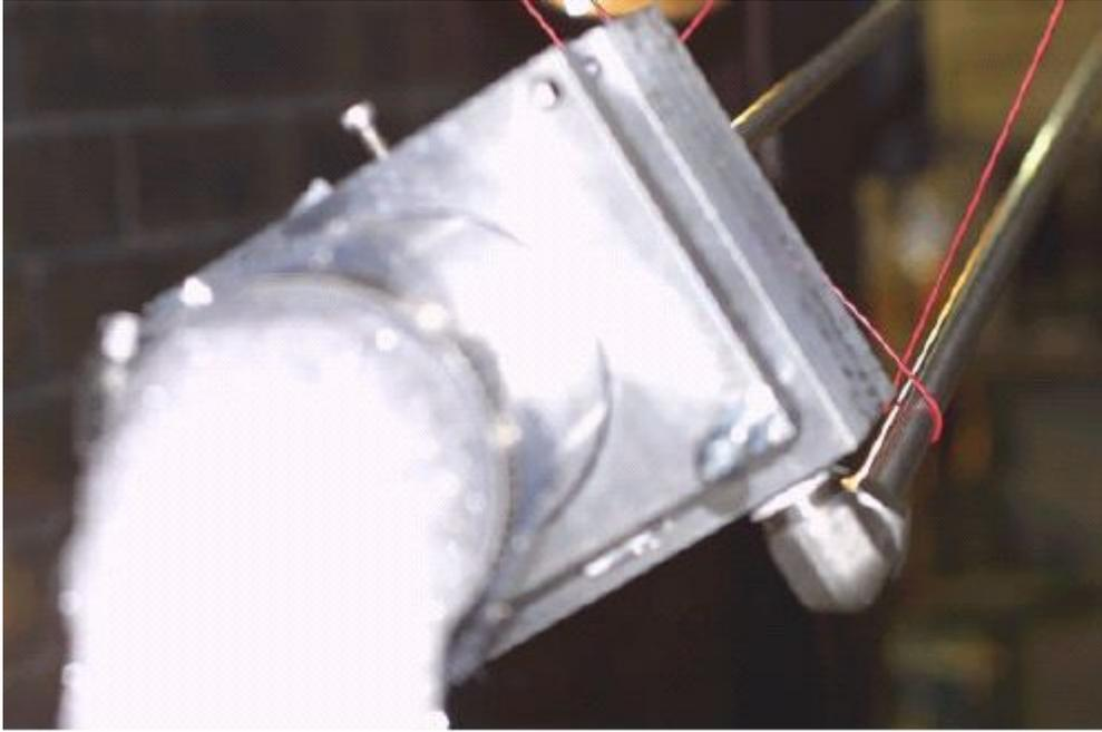
Figure 4: Foam Generator (front view, generating foam)
