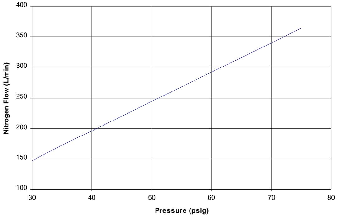
Figure 34: Nitrogen Flow Chart For 7/64-inch Opening in Nitrogen Line at the Device
