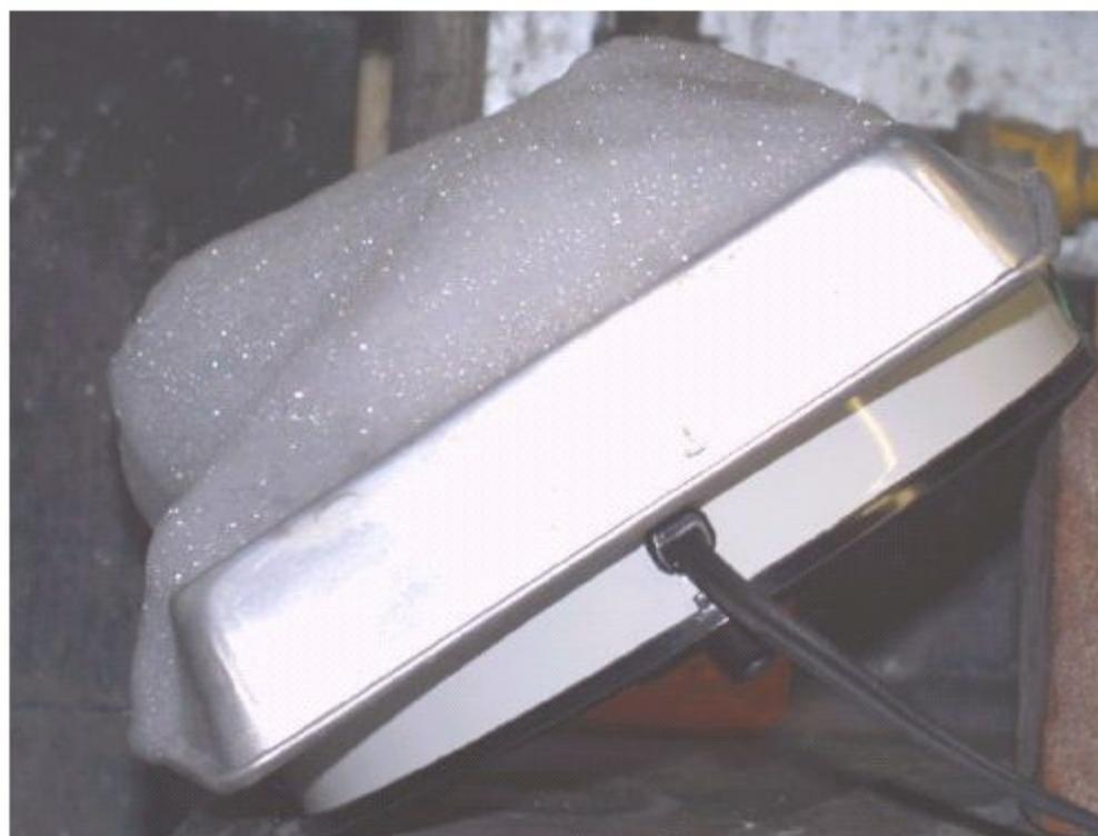
Figure 26: Hot Plate with Foam Applied: Expansion Ratio = 220
