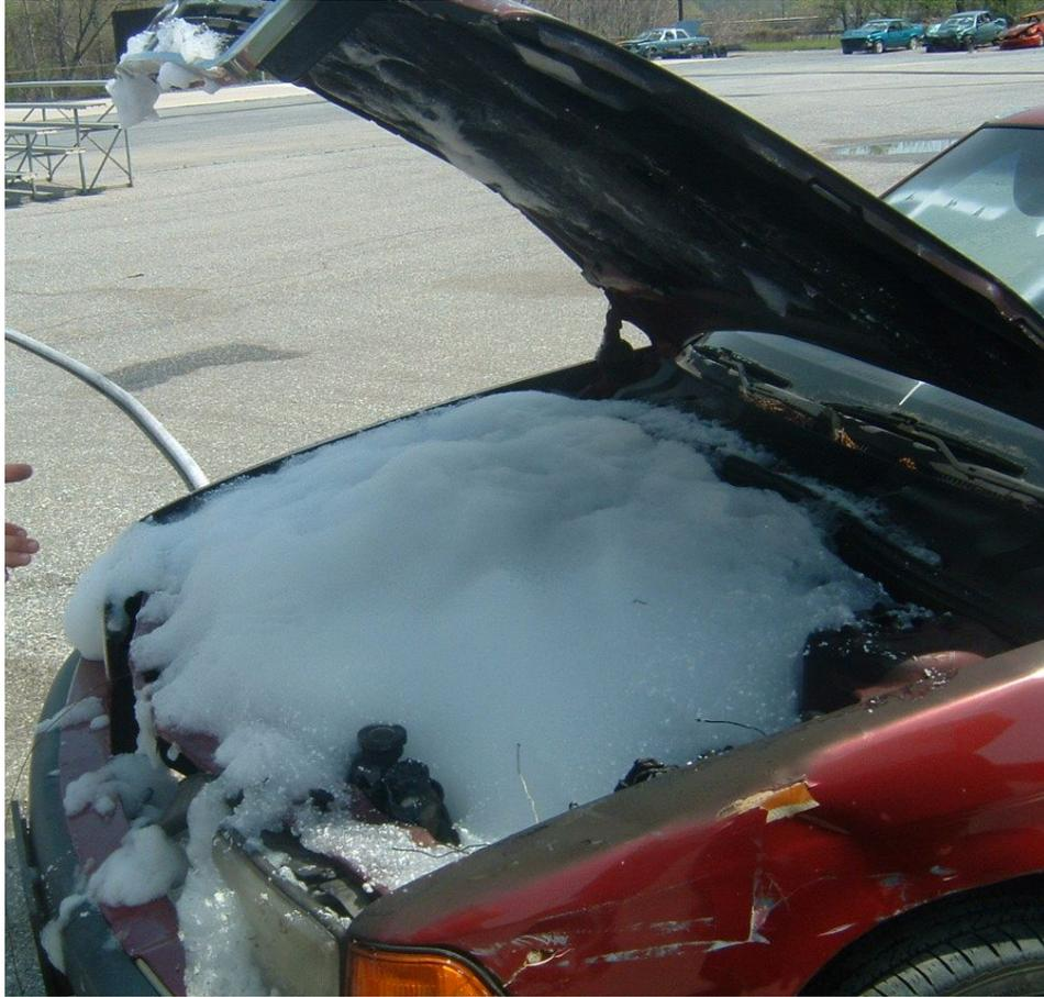
Figure 56: Foam Filled Chrysler Engine Compartment After 10 Minutes
