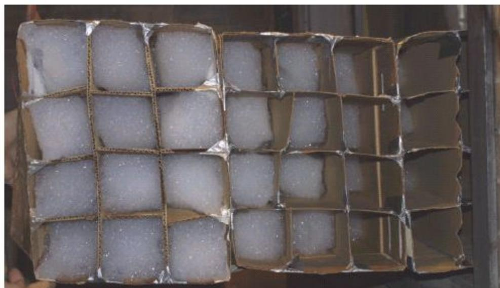
Figure 19: Box Set-Up #1 w/ 120 Expansion Ratio Foam
