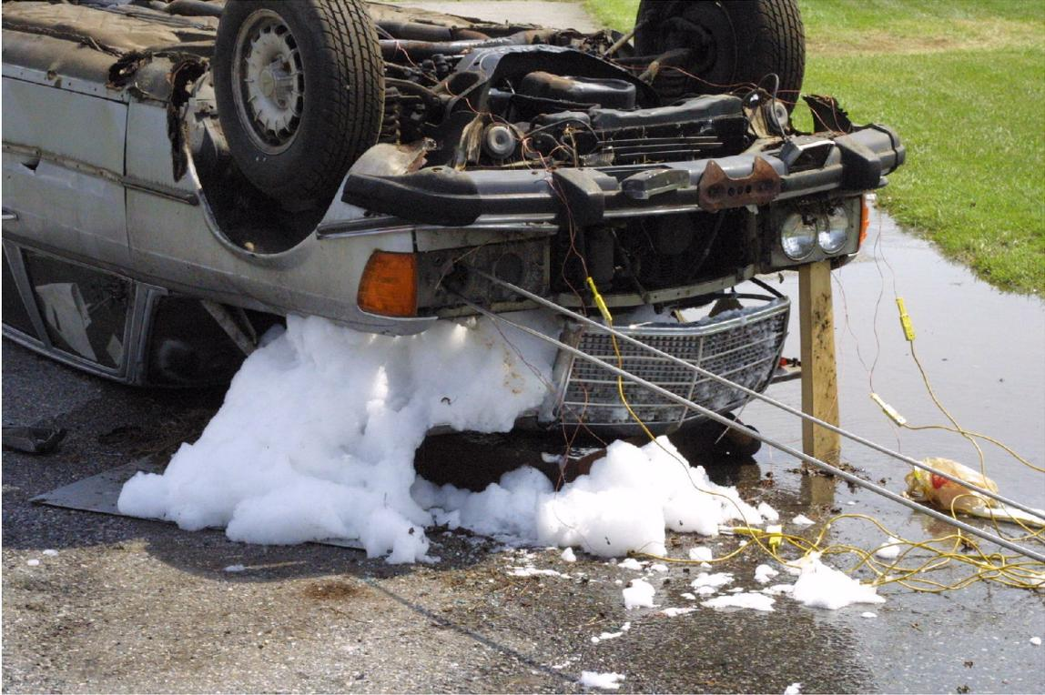
Figure 65: Movement of Foam from Sides of Hood.
