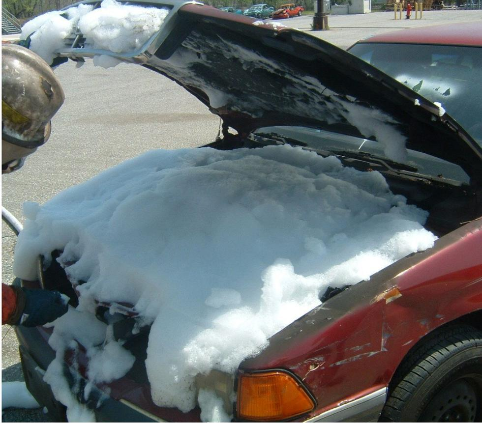
Figure 55: Foam Filled Chrysler Engine Compartment
