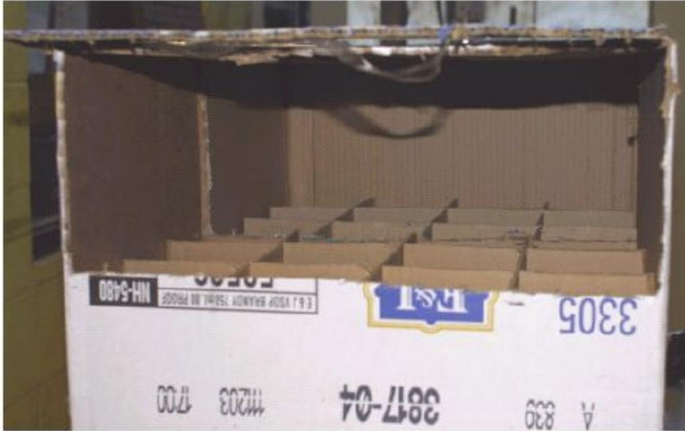
Figure 14: Inside View of Box for Modeling of Foam Flow in an Engine Compartment
