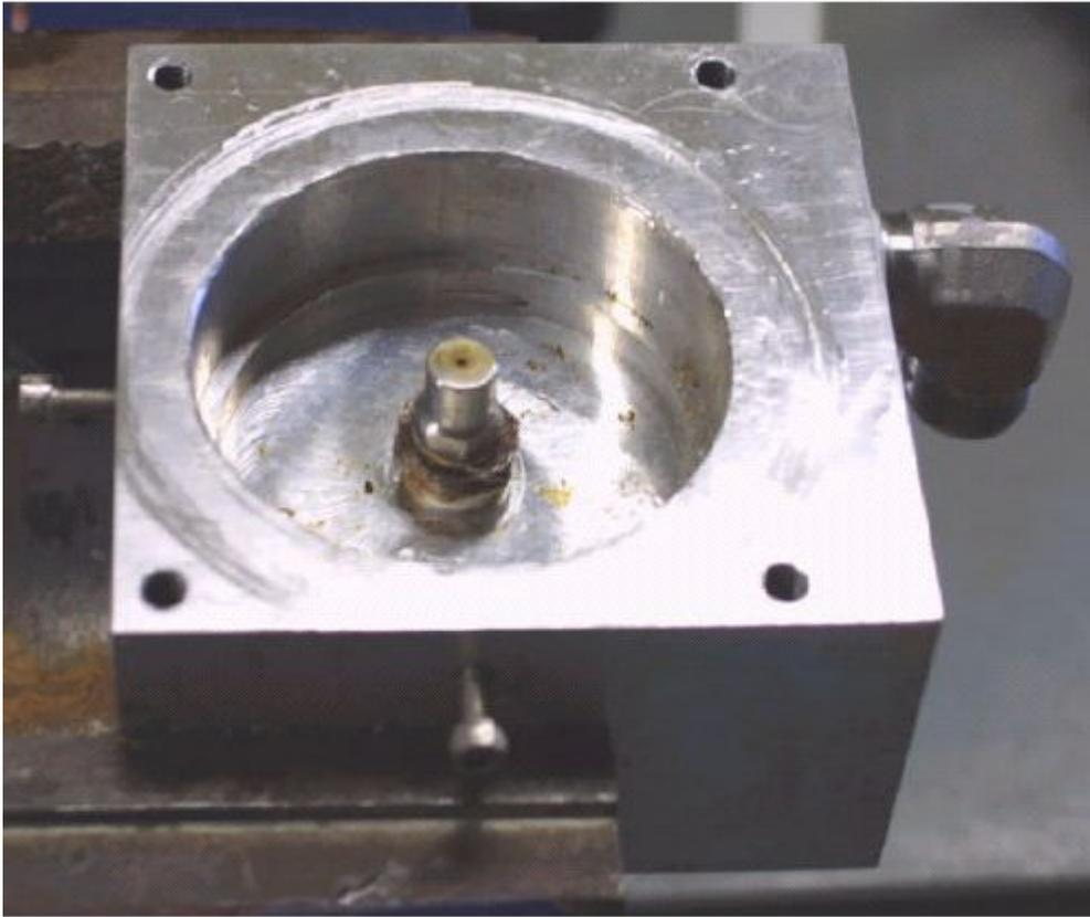
Figure 8: Foam Generator (top view) and Liquid Spray Nozzle
