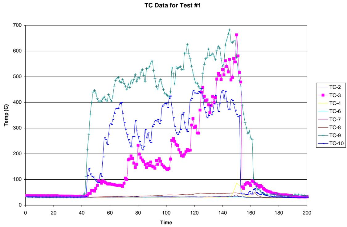
Figure 46: Thermocouple Data for Un-Suppressed Burn of Saturn
