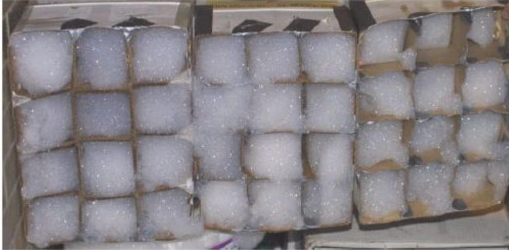
Figure 20: Box Set-Up #1 w/ 200 Expansion Ratio Foam
