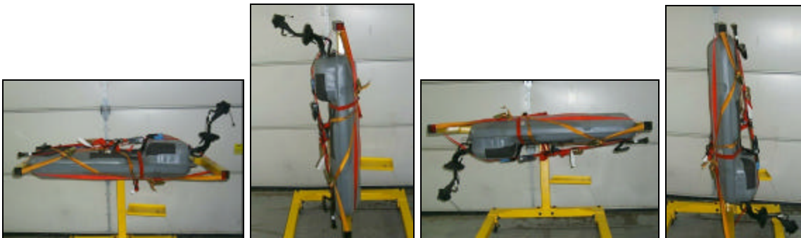
Figure 10: Typical test set-up for a leak test showing inversion of a tank system.
