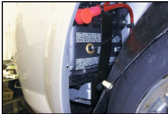
Figure 13: Sebring battery located in the front left bumper.
