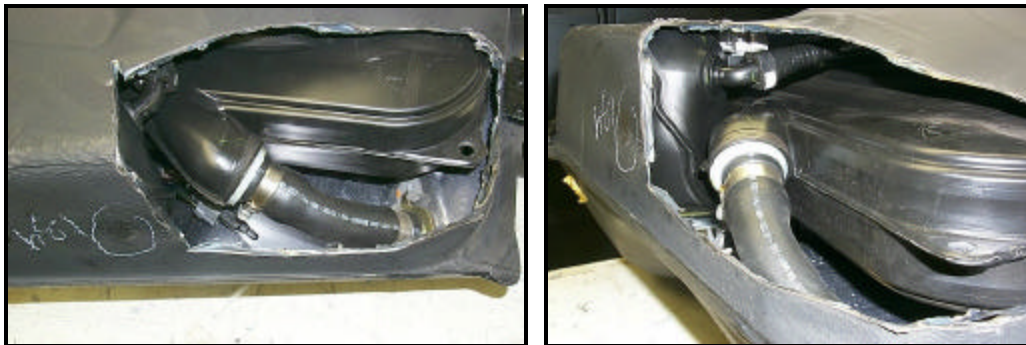
Figure 11: Cutaway view showing the plastic tank inside the steel outer shell of the Toyota Prius tank.
