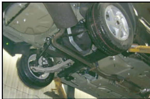
Figure 8: Typical over the axle tank placement.
