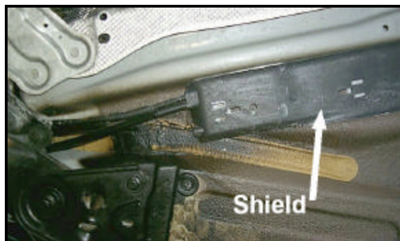
Figure 10: Partial fuel line shielding from a Volvo XC 90.
