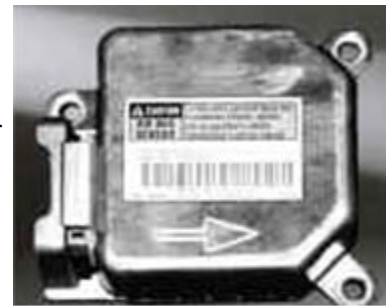
SCI studies emerging technology like the Airbag Sensing and Diagnostic Module (SDM).
