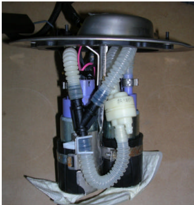
Figure 41: Ford Mustang sending unit.
