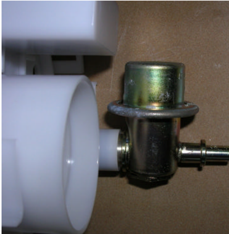
Figure 55: Kia Spectra fuel return valve.
