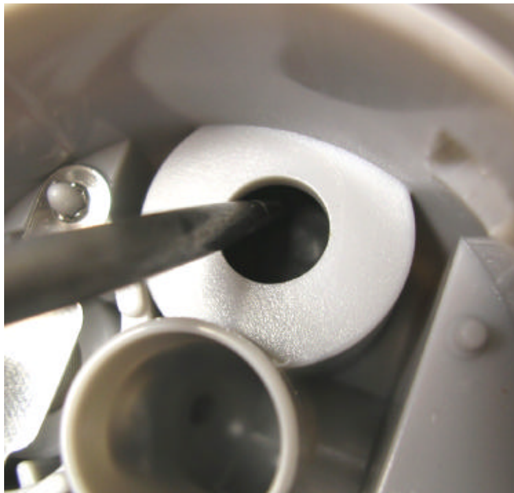
Figure 61: Kia Spectra fuel vapour port - one way valve.
