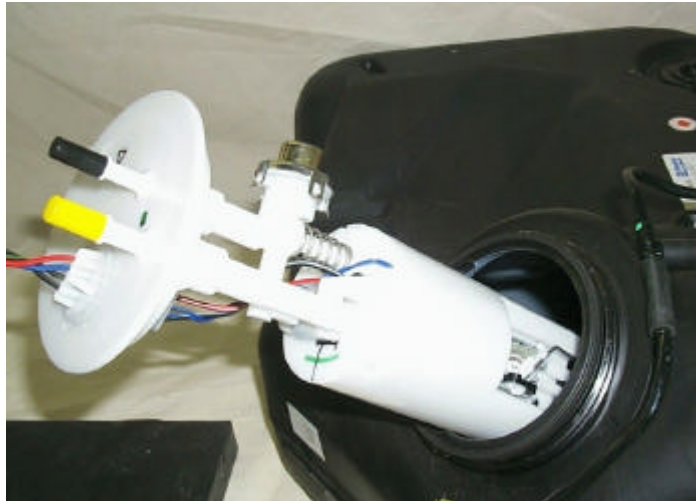
Figure 18: Chrysler Cirrus sending unit.
