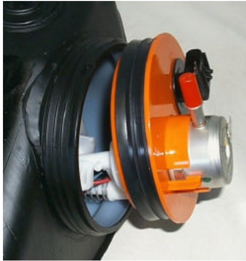
Figure 30: Dodge Neon sending unit.
