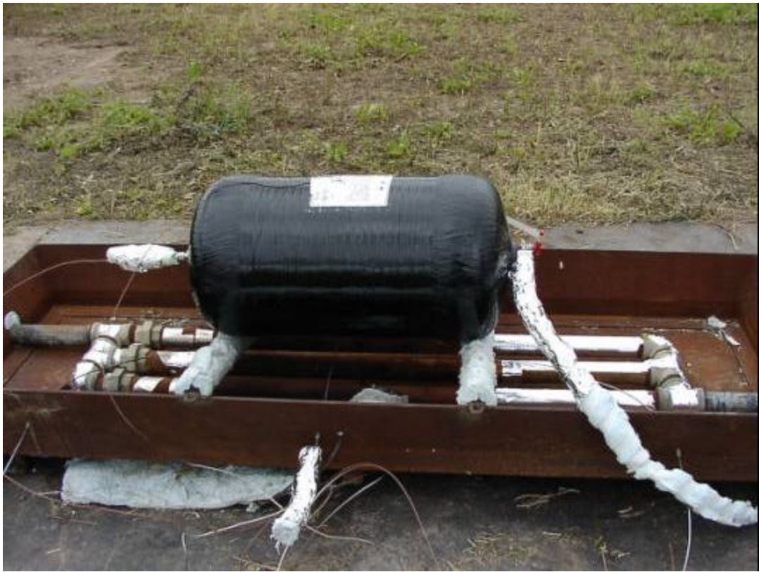
Figure B-1. Type -IV Hydrogen Cylinder Located on Bonfire Source.
