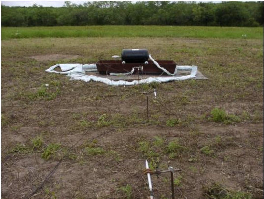
Figure B-2. View of Blast-Wave Pressure Transducers on West Side of Cylinder.
