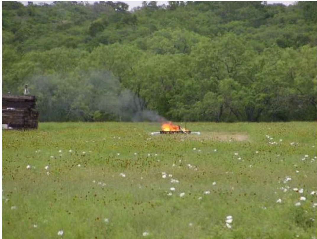
Figure B-4. Cylinder Under Bonfire. Note soot from combustion of cylinder materials.
