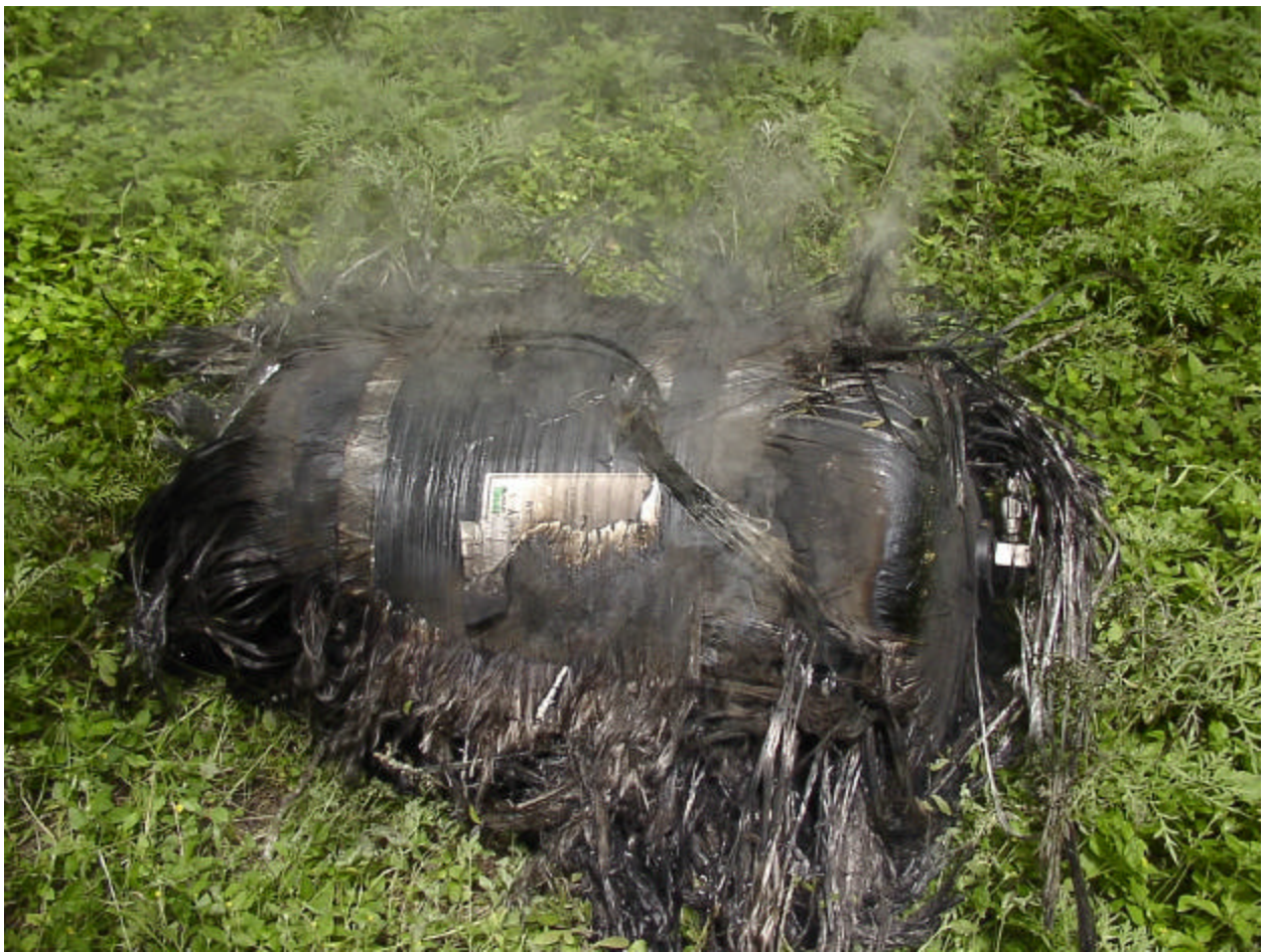
Figure B-7. Main Portion of Cylinder Remains.
