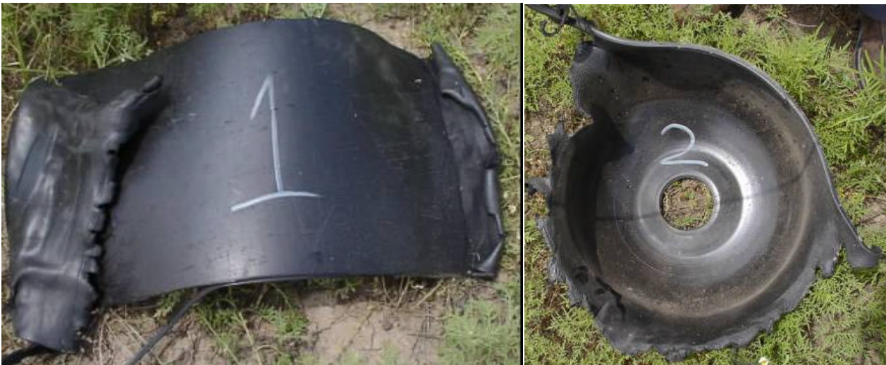
Figure B-8. Main Cylinder and Dome of Polyethylene Liner.
