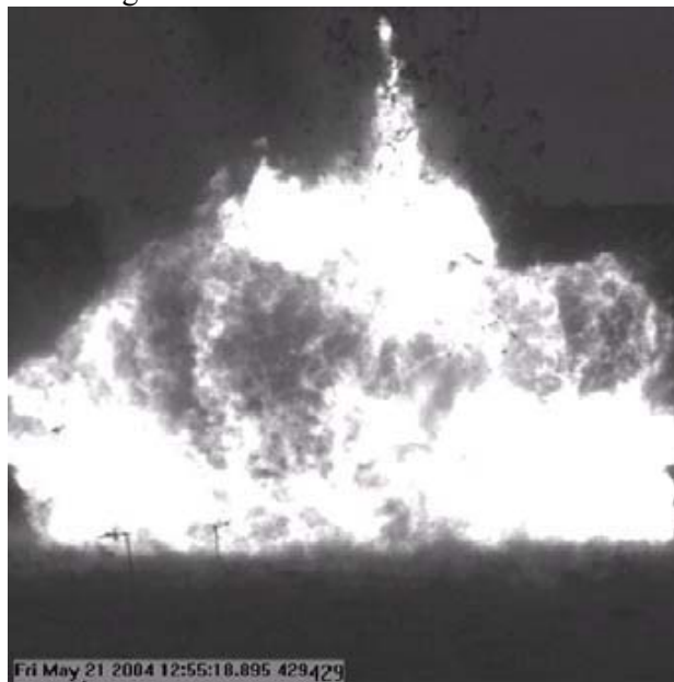
Figure 7a Fireball 45 msec after tank rupture in Test 1.
