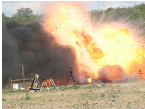
Figure 8b. Hydrogen fireball about 170 msec after tank rupture in Test 2.
