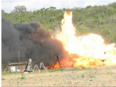
Figure 8a. Hydrogen fireball about 70 msec after tank rupture in Test 2.
