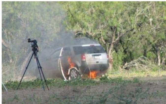
Figure 4a. SUV and tank fire exposure and spread to left rear wheel-well at about 2 minutes.
