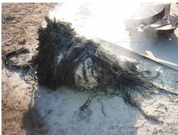
Figure 11. Large tank fragment from Test 2.
