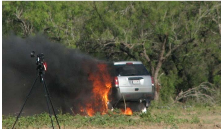
Figure 4c. SUV and Type 3 tank after about 9 minutes of exposure fire.
