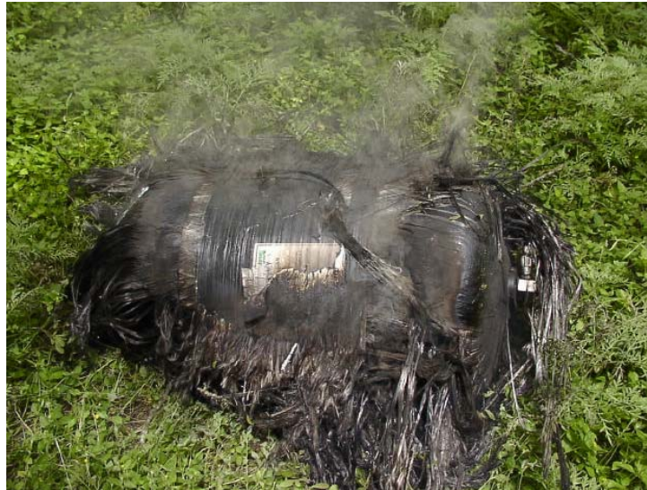
Figure 9. Large fragment from cylinder in Test 1.
