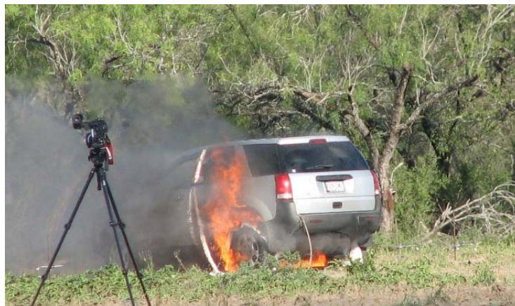
Figure 4b. SUV and tank after about 4 minutes of exposure fire.
