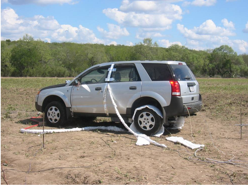
Figure 2 Instrumented SUV with Type 4 Hydrogen Fuel Tank
