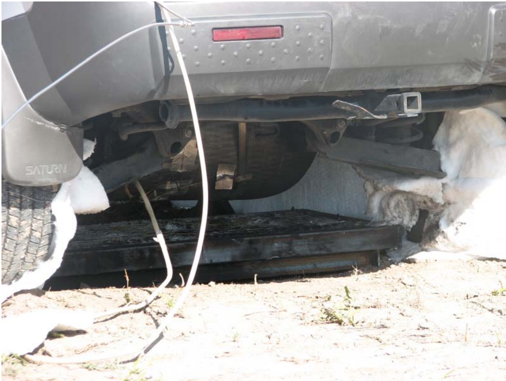
Figure 3 Type 4 Fuel Tank Mounted on SUV and over Propane Burner
