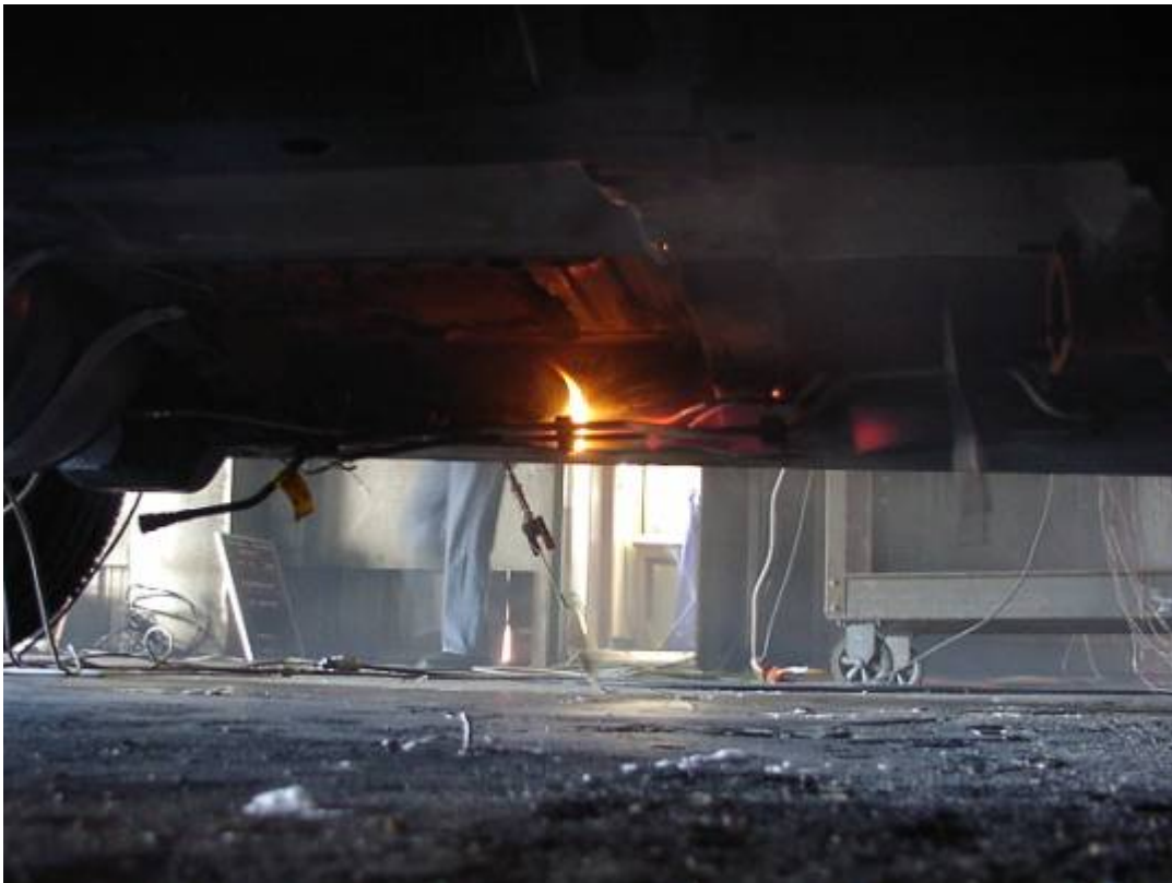
Figure F-12. Continued Flaming of Plastic Component, Glowing Metal Components.
