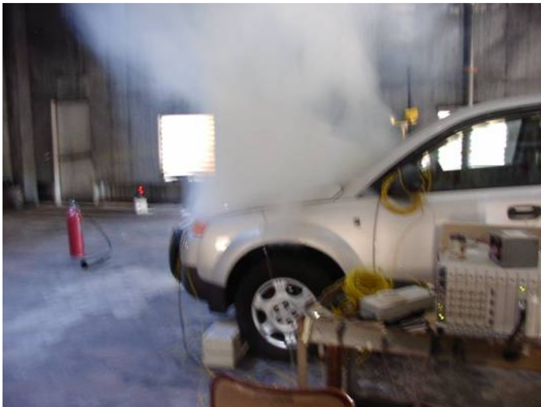
Figure F-8. Effects of Jet-Fire With Hood Closed.
