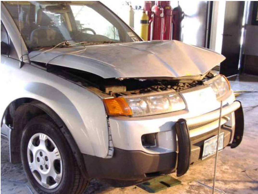
Figure 6. 64-Sec Duration Test – Damage to Hood Following Series 2 Tests.
