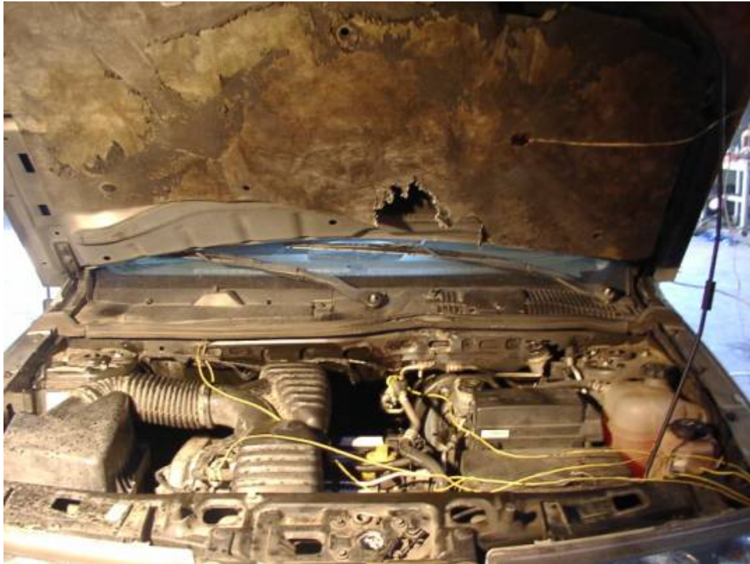
Figure F-9. Damage to Underside of Hood Liner Following Series 4 Tests.
