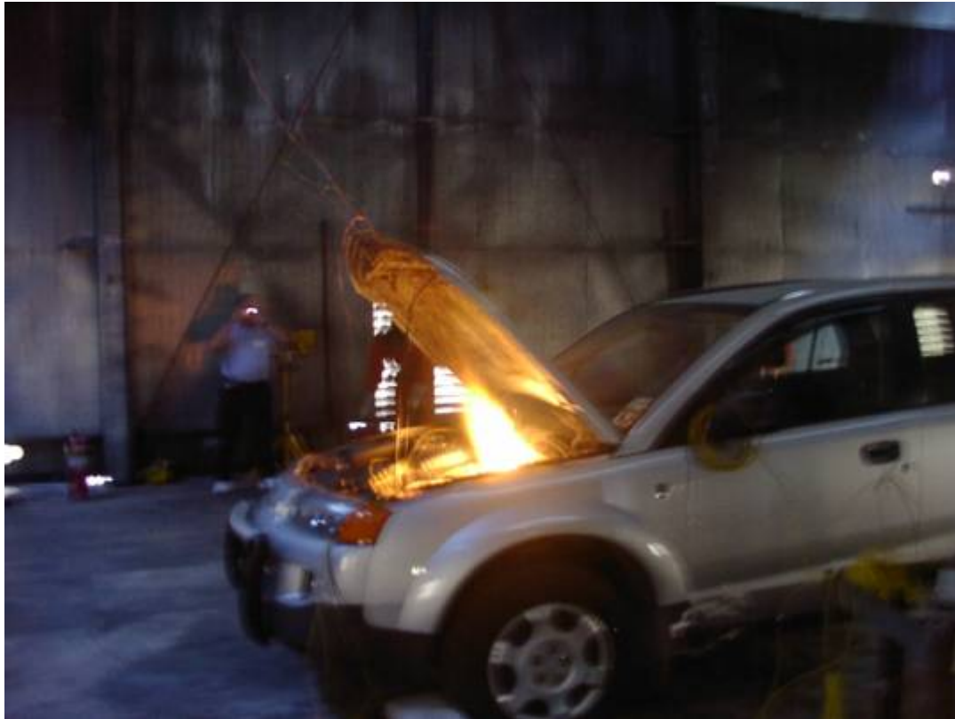
Figure F-7. Jet-Fire Length During Open Hood Test.
