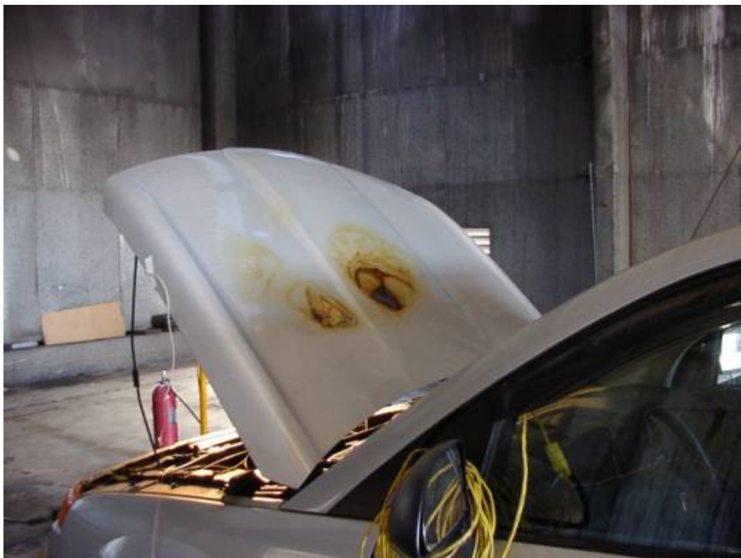
Figure F-10. Damage to Topside of Hood Following Series 4 Tests.
