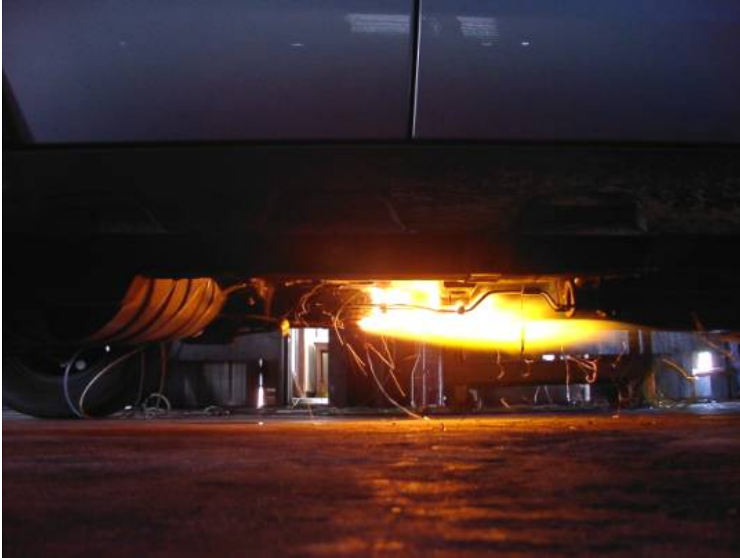
Figure F-11. View of Jet-Fire on Underside of Vehicle.
